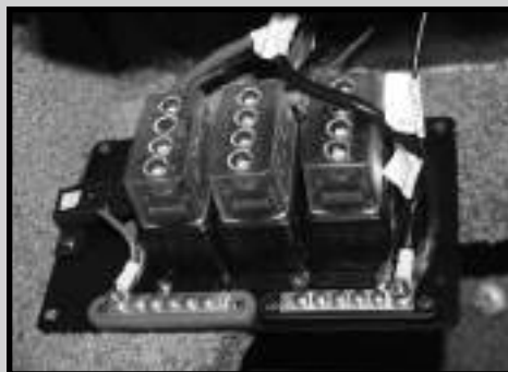
Fuse Panel - Under Dash
