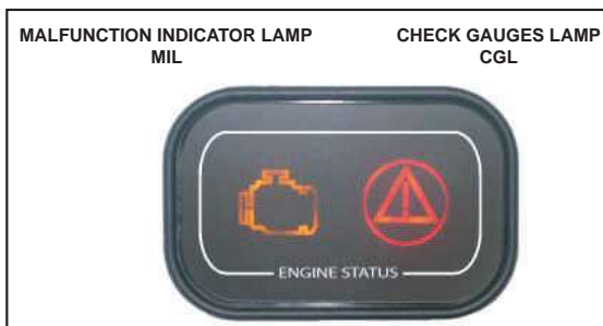
Figure 5-1A Example Warning Lamp Cluster
