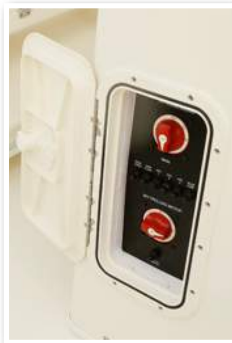
Battery Switch, Shown in the "Off" Position
