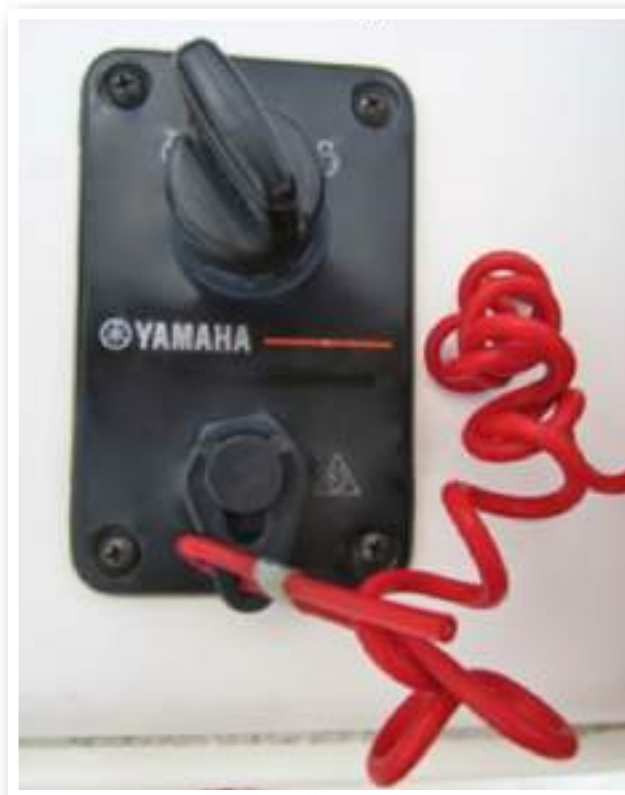
Engine stop switch (above)
