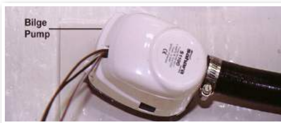
The Bilge Pump is Mounted to ABS Plastic
