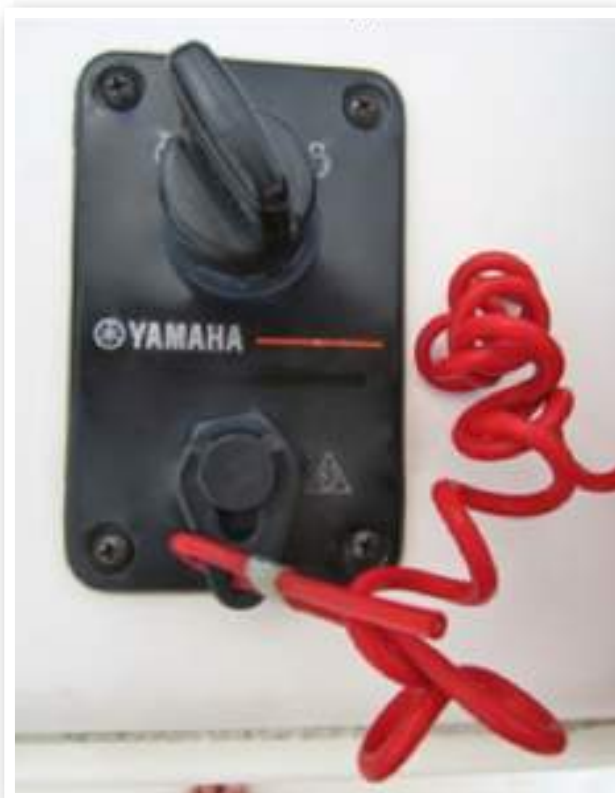
Engine stop switch (above)
