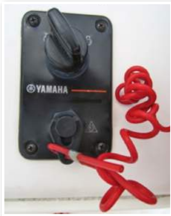
Engine stop switch (above)
