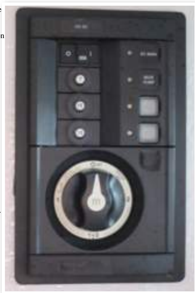
Battery Switch, Shown in the "Off" Position
