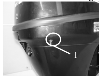
1. Cooling water checking hole
