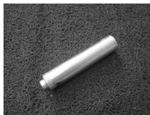
Lower casing cover oil seal installer
