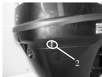
2. Cooling water checking hole
