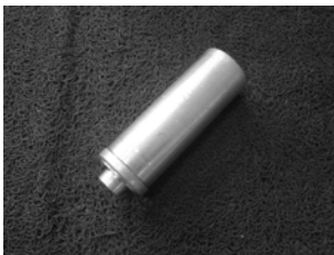
Lower casing cover bearing installer
