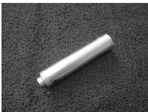
Lower casing cover oil seal installer
