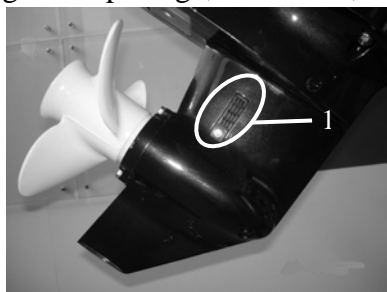
1. Cooling water passage inlet
