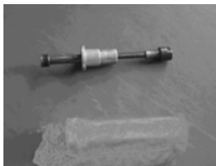
Barrel bearing with guard board installer tool
