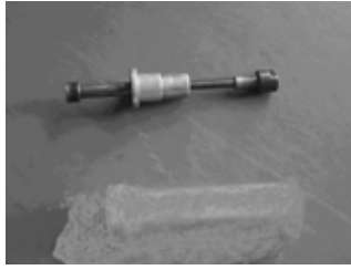
Barrel bearing with guard board installer tool
