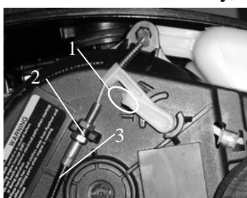
1. Triangle marking 2. Adjusting nut 3. Tightwire ass'y, detent
