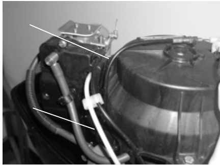
1. Start-in-gear protection device cable 2. Chock lever cable
