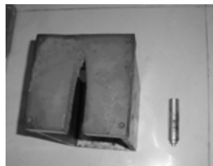
Lower casing bracket and sleeve bearing without guard board installer tool
