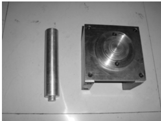
Housing bearing installer
