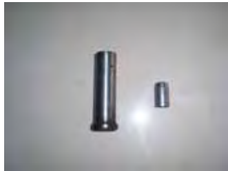
Housing oil seal installer
