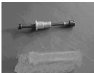
Sleeve bearing with guard board installer tool
