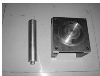
Housing bearing installer
