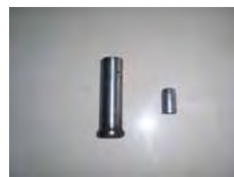
Housing oil seal installer
