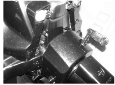
1. Cooling water checking hole
