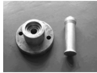
Lower casing cover bearing installer
