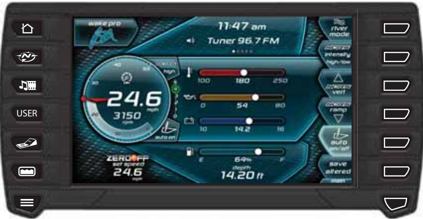
HOME menu for LINC with NCRS (the second set of soft keys is displayed)
