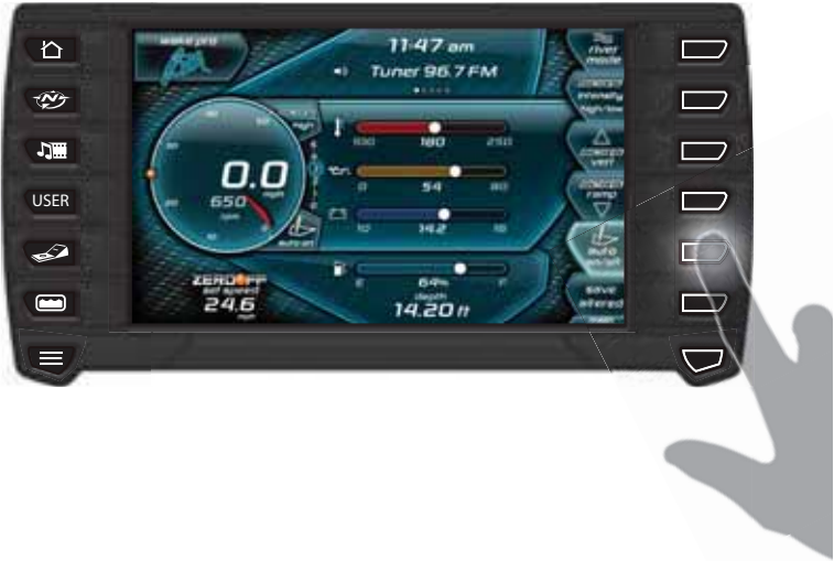
HOME menu for LINC with NCRS (the second set of soft keys is displayed)
