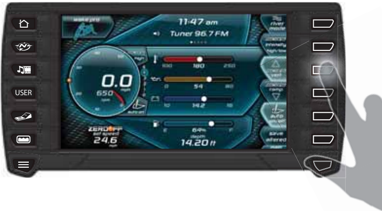
HOME menu for LINC with NCRS (the second set of soft keys is displayed)
