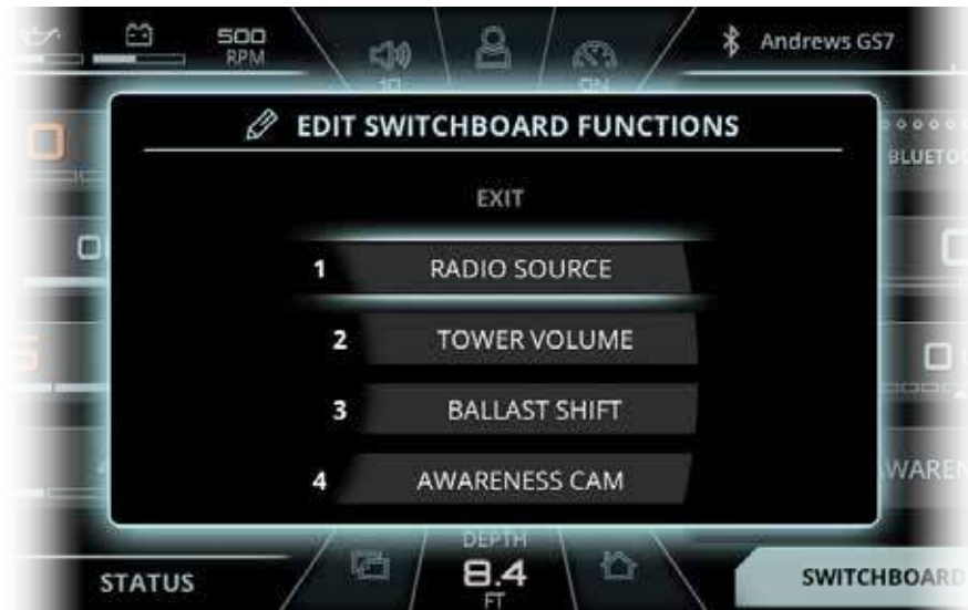
FIG. P2- SWITCHBOARD TAB ON THE RIGHT SECTION OF THE DISPLAY
