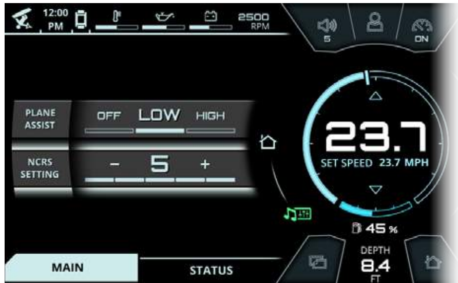
FIG. C1 - MAIN TAB ON THE HOME MENU, WAKEBOARD SPEED (G AND GS MODELS)
