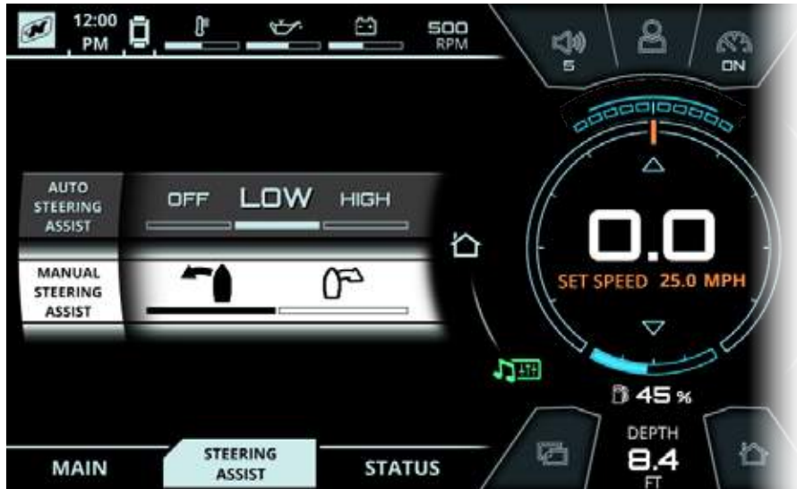
FIG. F3 - MANUAL STEERING, BOW PORT SELECTED. THRUSTER IS IN USE (BLUE GRAPHICS)
