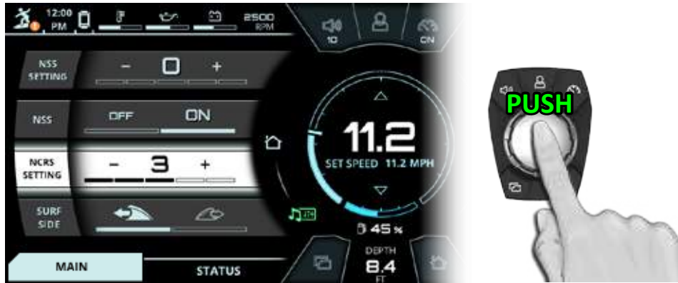
FIG. A8 - PUSHING DOWN TO SELECT A SETTING (THE NCRS SETTING IN THIS EXAMPLE)
