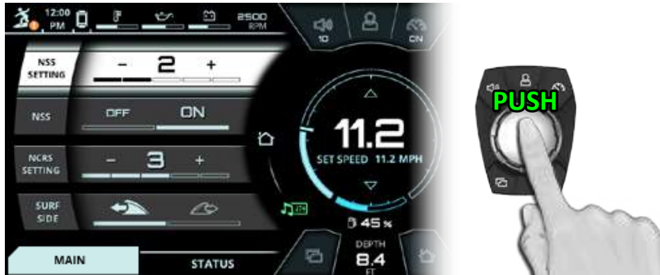
FIG. A4 - PUSHING DOWN TO SELECT A SETTING (THE NSS SETTING IN THIS EXAMPLE)
