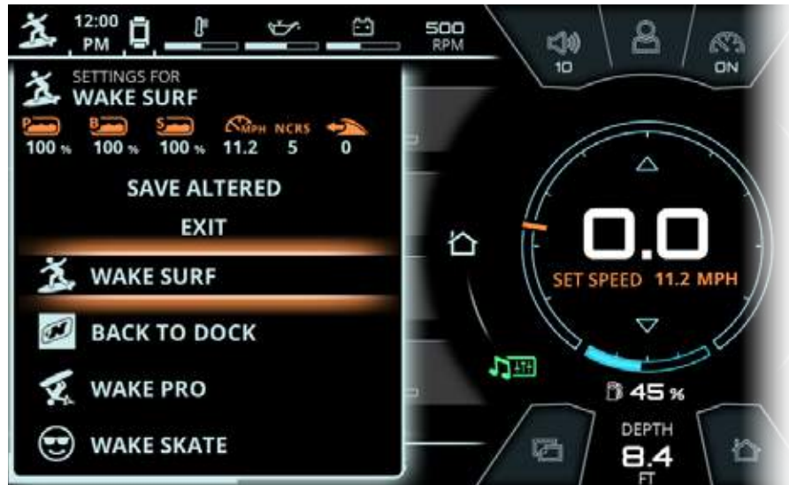
FIG. B2 - DROP-DOWN MENU AFTER PRESSING THE USER BUTTON ON HELM COMMAND
