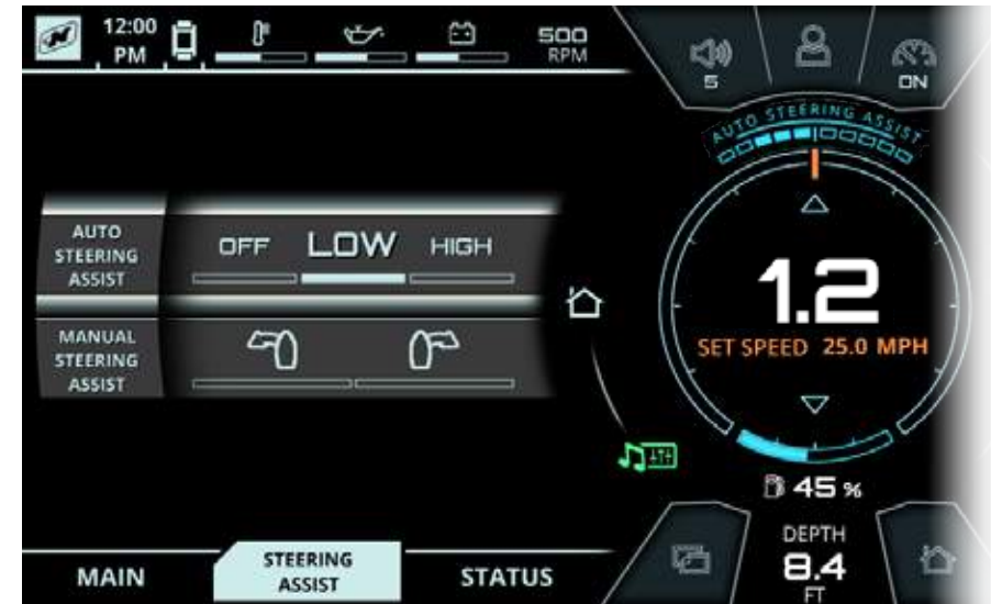
FIG. F2 - AUTO STEERING ASSIST SET TO LOW AND THRUSTER IN USE (BLUE GRAPHICS)
