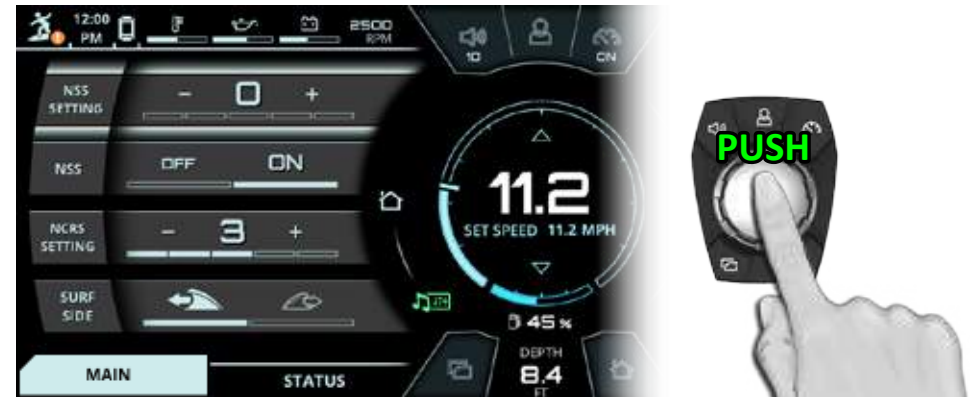
FIG. A6 - PUSHING DOWN TO DE-SELECT A SETTING (THE NSS SETTING IN THIS EXAMPLE)
