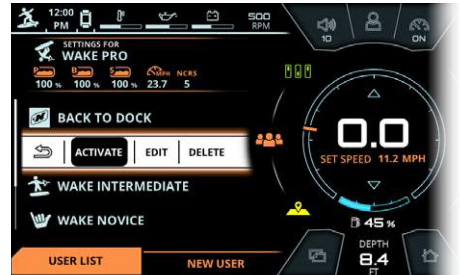
FIG. L2 - USER LIST TAB ON THE USER MENU (WITH A USER PROFILE IN THE SELECTED STATE)
