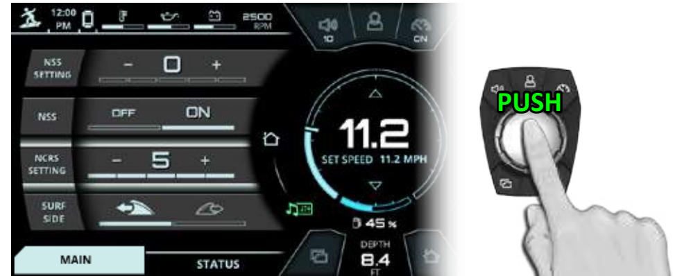
FIG. A10 - PUSHING DOWN TO DE-SELECT A SETTING (THE NCRS SETTING IN THIS EXAMPLE)
