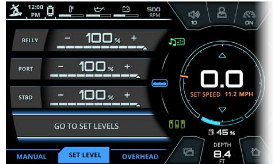
FIG. J2 - SET LEVEL TAB ON THE BALLAST MENU
