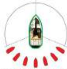
You are the privileged vessel being overtaken. Red boats are burdened vessels overtaking.
