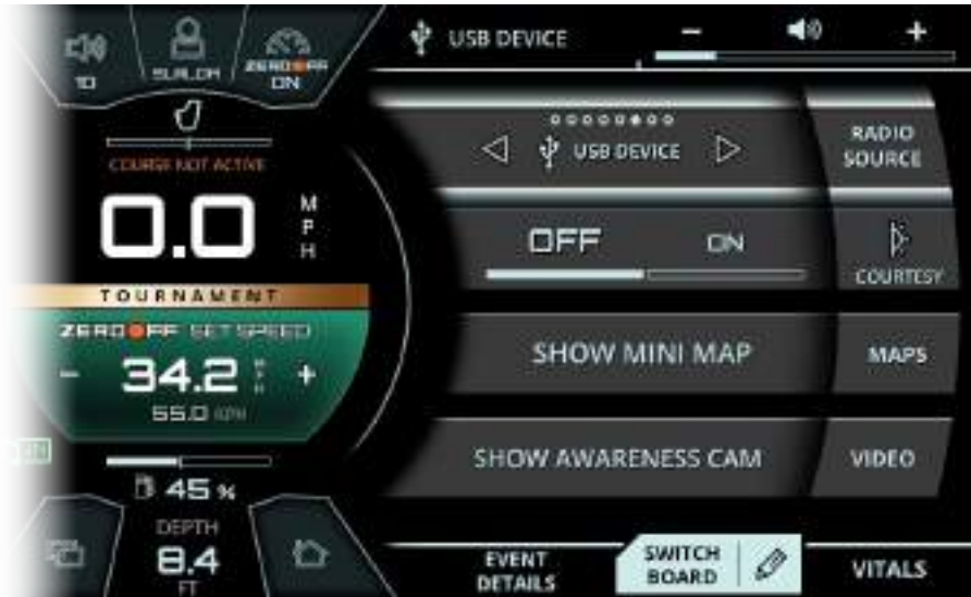
FIG. D3 - SWITCHBOARD TAB ON THE RIGHT SECTION OF THE SCREEN
