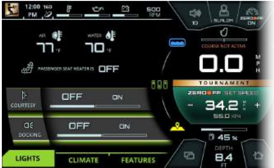
FIG. J1 - LIGHTS TAB* ON THE SWITCHING MENU
