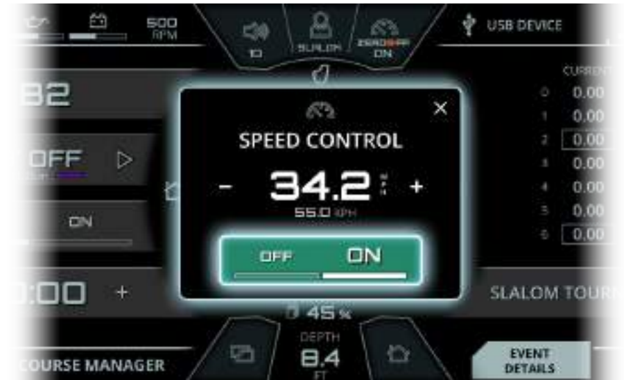
FIG. B3 - POP-UP AFTER PRESSING THE SPEED CONTROL BUTTON ON HELM COMMAND
