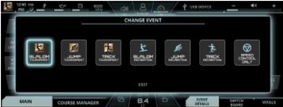
FIG. B2 - POP-UP AFTER PRESSING THE CHANGE EVENT BUTTON ON HELM COMMAND
