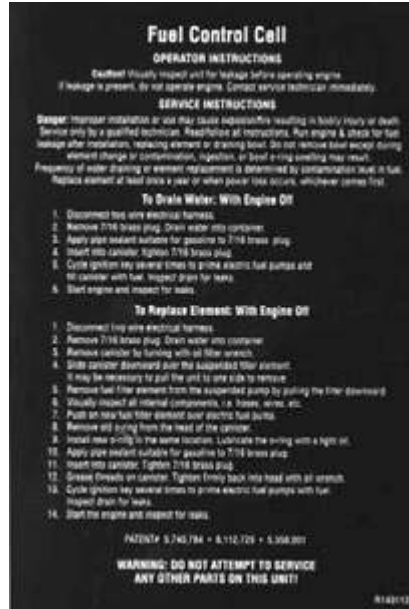
Fuel Control Cell
