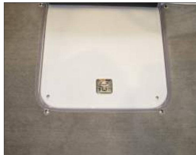
Typical Twist Lock Latch - Latched With Handle Folded Flush
