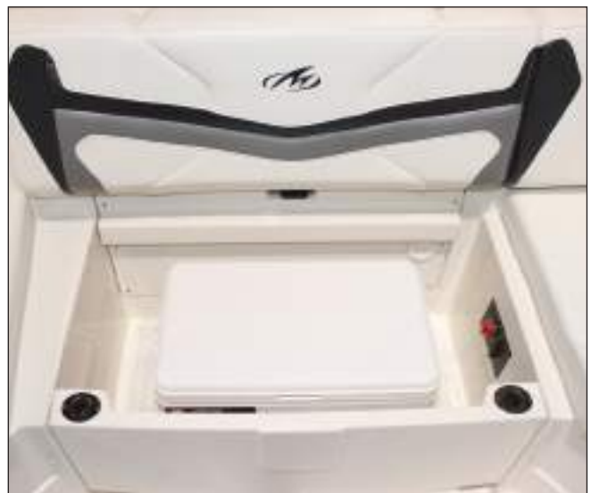
Cooler/Battery Switch/Fire Port Compartment 214SS/218SS & 234SS/238SS
