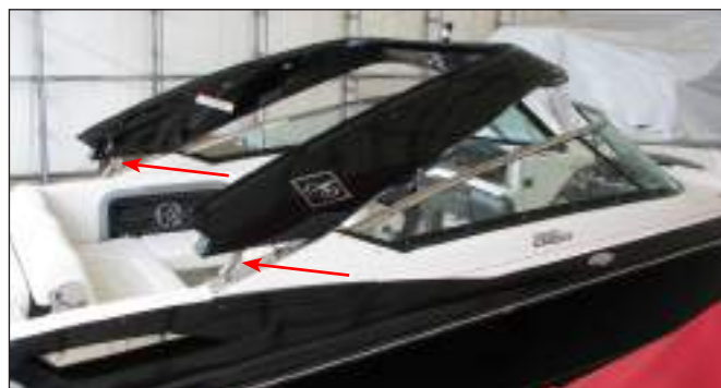
Fiberglass Electric Folding Arch & Actuators
