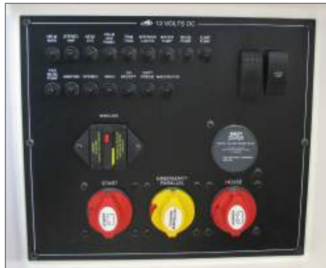
288SS Battery Switch Panel, Circuit Protection & Switches
