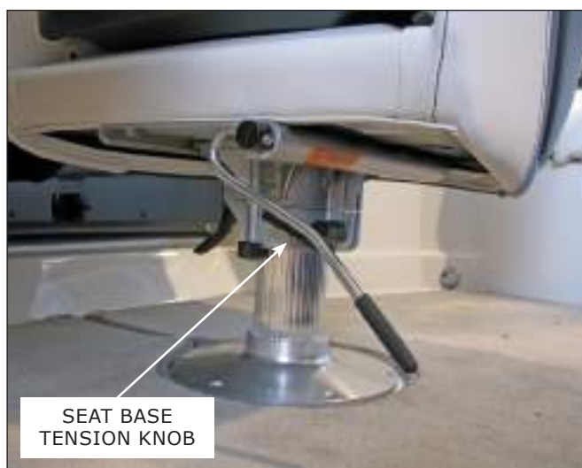
Helm & Passenger Seat Base Adjustment Levers
