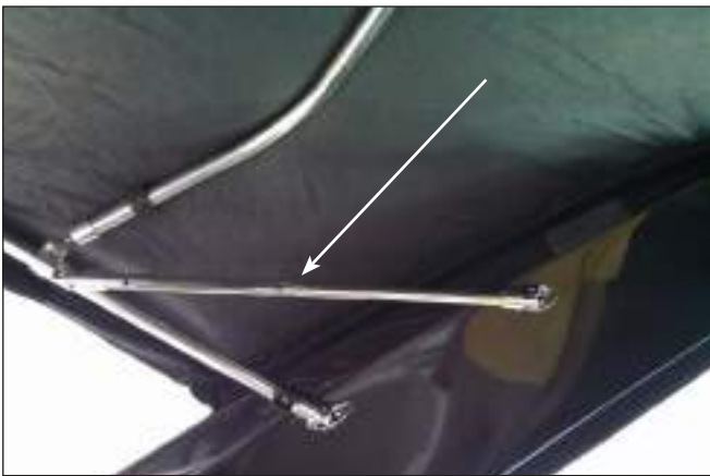
Adjustable Stanchion Supporting Rear Top Section
