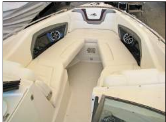
288SS Bow Seating Area - Filler Cushions Installed
