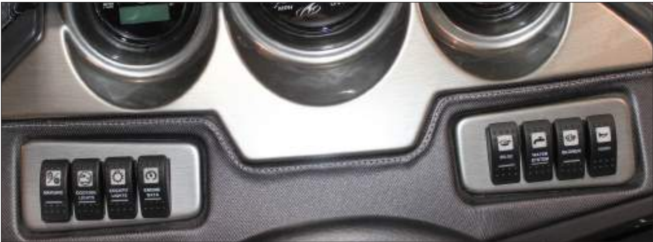
Helm Switch Panels 214SS/218SS & 234SS/238SS
