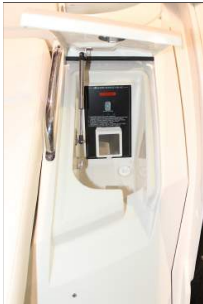
328SS Shore Power Inlet Panel
