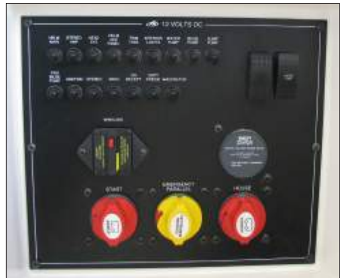
288SS Dual Battery Switch Panel & Circuit Protection
