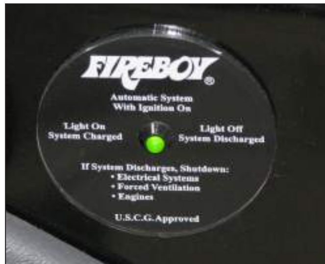
Fire Extinguisher Panel In Helm
