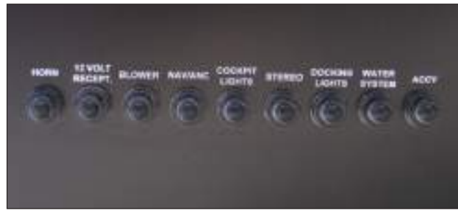
Helm Accessory Circuit Breaker Panel 214SS/218SS & 234SS/238SS
