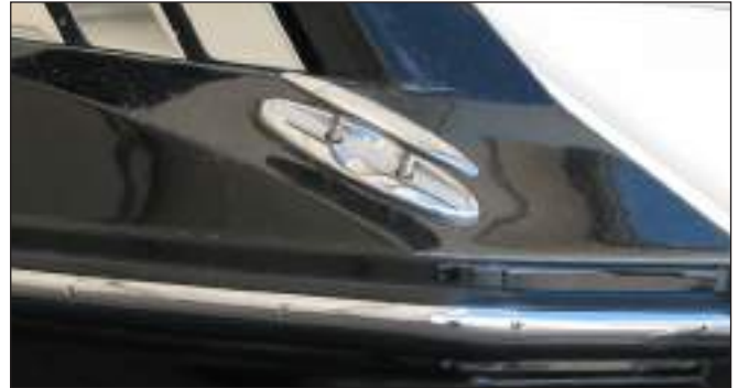
Retractable Cleat Deployed
