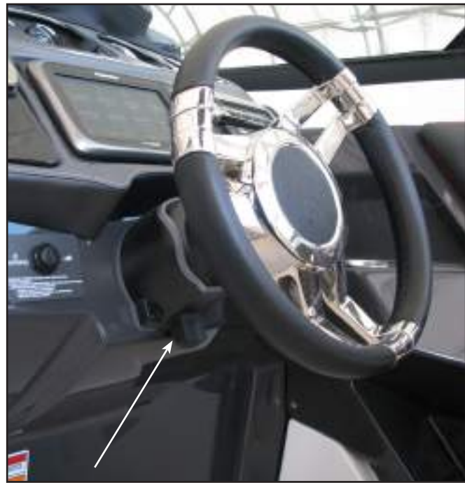
Tilt Steering Wheel & Tilt Release Lever
