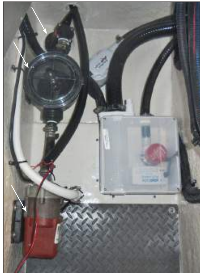
Typical 120-Volt Air Conditioner Pump, Strainer & Thru-Hull Valve
