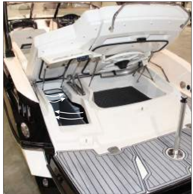
288SS Engine Compartment Air Flow Through Storage Compartment
