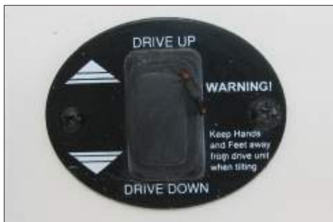
Typical Outdrive Tilt Switch Near Transom Door
