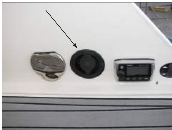
AC Battery Charger System Inlet Connection
