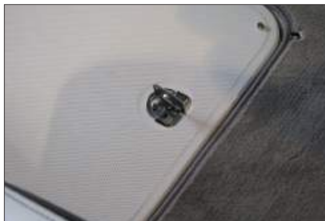
Typical Twist Lock Latch - Not Latched With Handle Up
