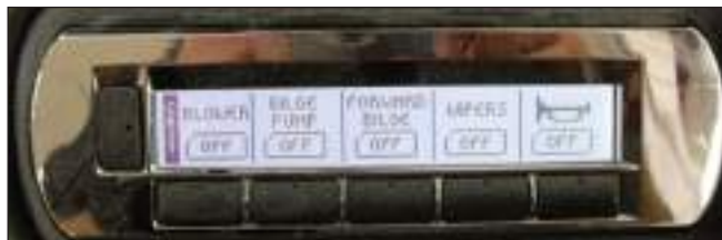
Critical Page - Digital Switch Panel
