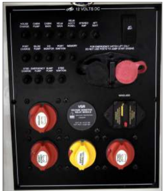
328SS Battery Switch Panel, Circuit Protection & Switches
