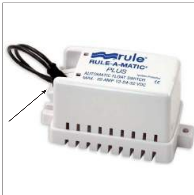
Emergency Pump Automatic Float Switch Test Button Push Button Down & Hold Until Pump & Alarm Activate
