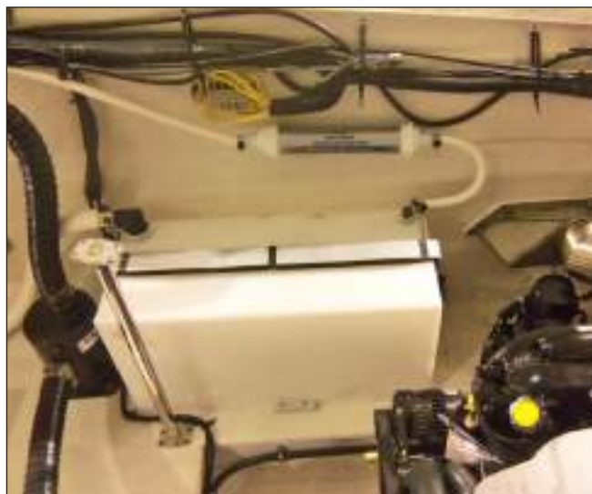
328SS Holding Tank & Charcoal Filter
