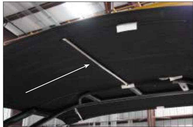
Center Adjustable Stanchion Supporting Rear Top Section
