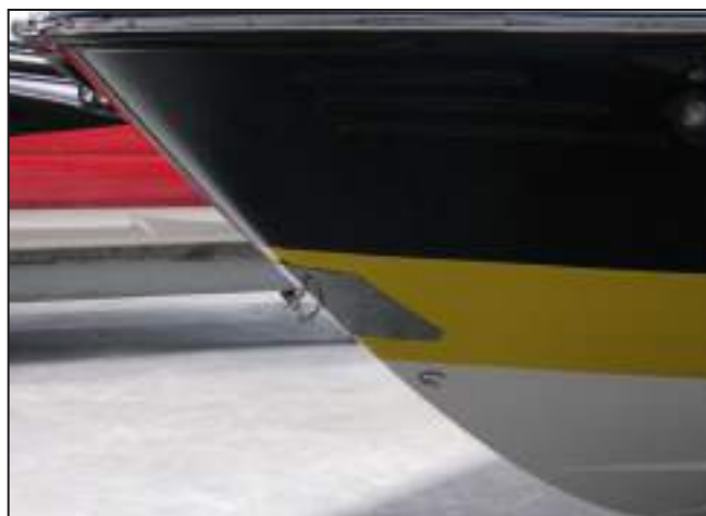
Typical Rope Locker Drain
