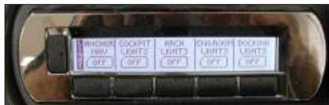
Lights Page - Digital Switch Panel
