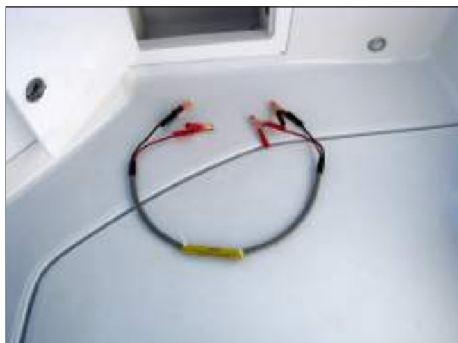
Emergency Aft Cockpit Hatch Jumper Harness
