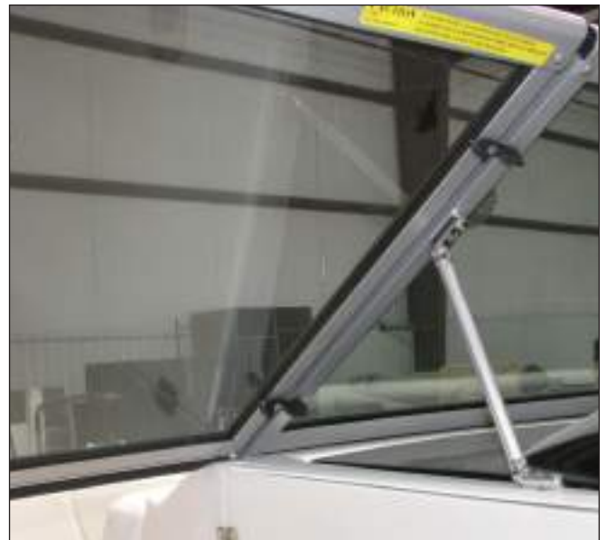
Typical Windshield Center Section Latches (The latches and windshield frame shown may be slightly different than your boat and are for reference only)
