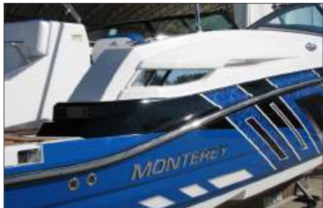
Bilge Compartment Vents
