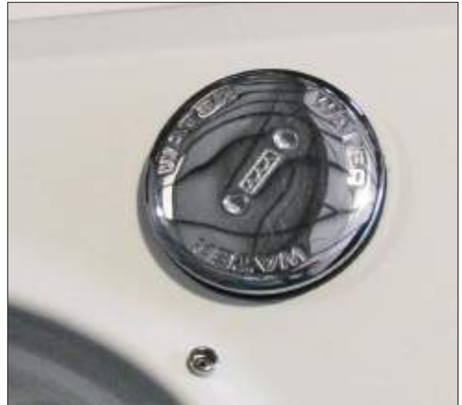
Fresh Water Fill
