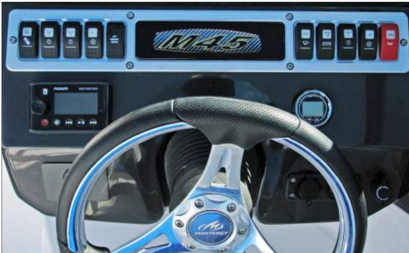
Helm Switch Panels
