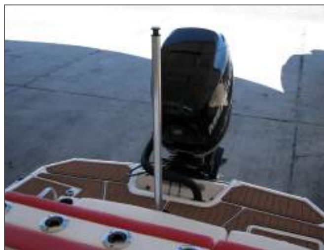
Ski Tow Pylon
