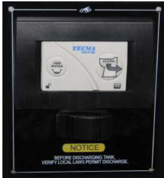
Electric Head Control Panel In Head Compartment
