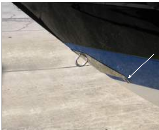
Rope Locker Drain
