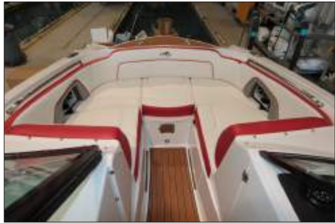
M-45 Bow Lounge Seat Cushions Installed & Foldout Supports Latched Open
