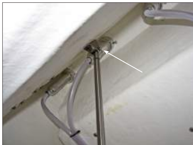
Aft Cockpit Hatch Actuator Emergency Quick Release Pin
