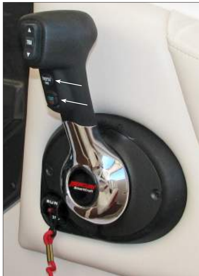
Typical Mercury Electronic Control & Switches
