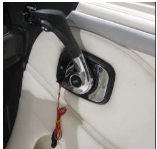
Typical Volvo Side Mount Cable Control & Stop Switch
