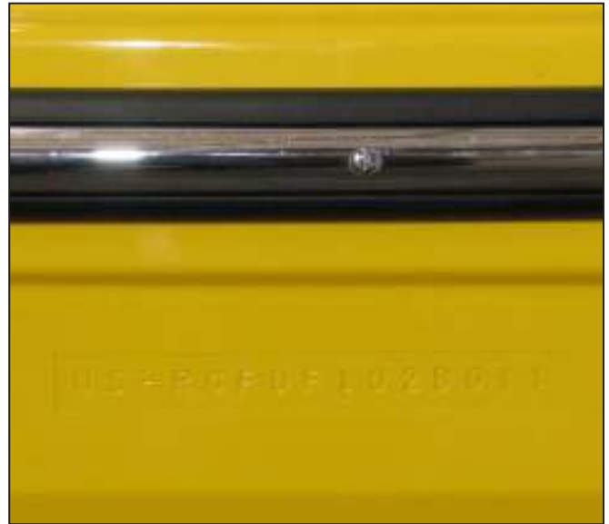
Hull ID # On Starboard Side of Transom
