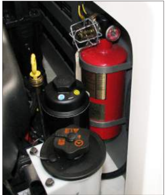
Typical Automatic Fire Extinguishing System In The Engine Compartment
