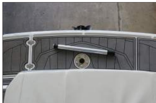
Ski Tow Pylon & Base
