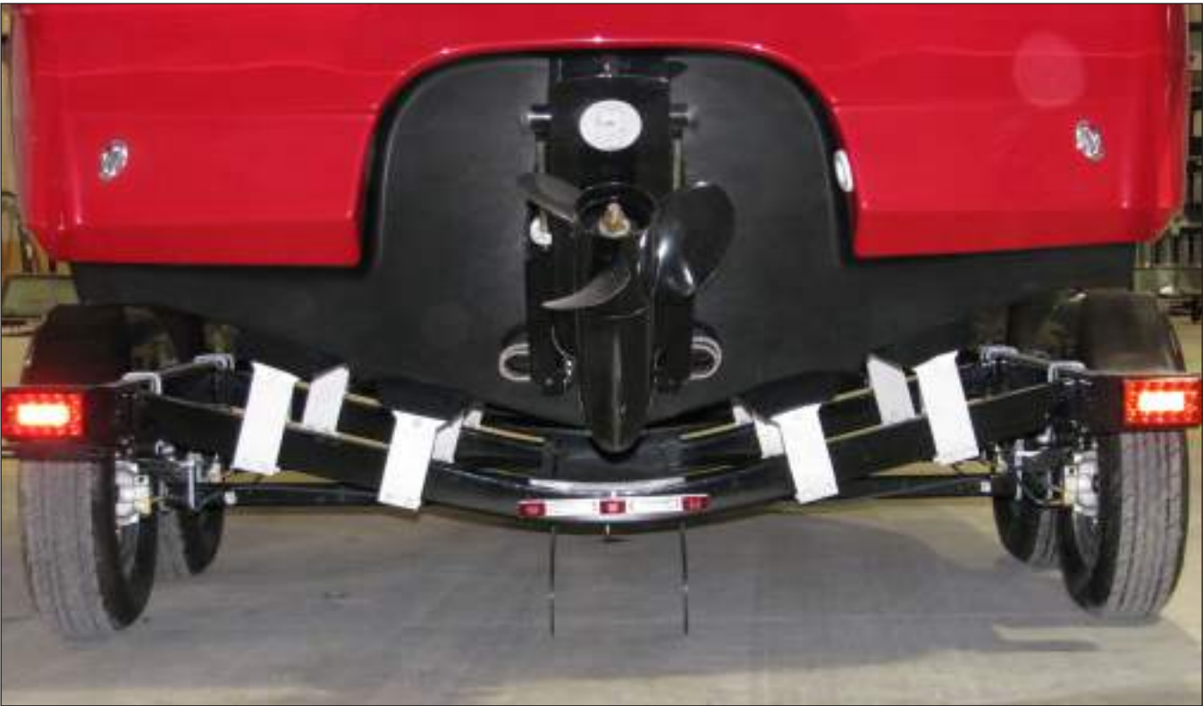
Trailer Bunks - Supporting Hull Properly
