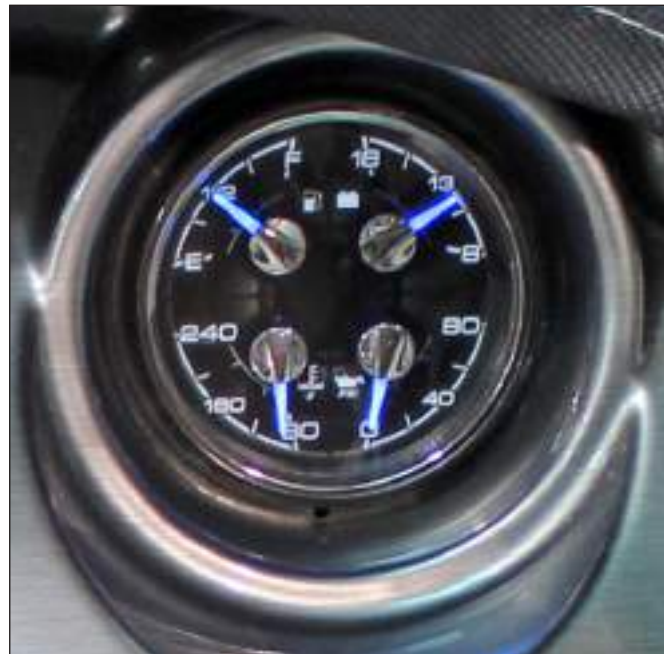
Typical Backlit Multi Gauge Fuel Level, Engine Temperature, Voltage & Oil Pressure
