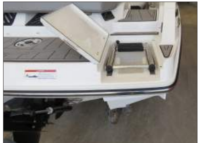
Boarding Ladder In Compartment
