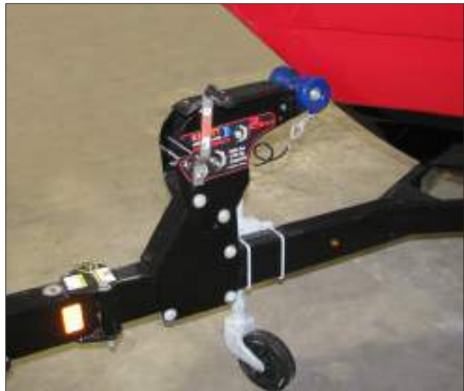
Bow Seated in Bow Roller with Safety Cable Attached
