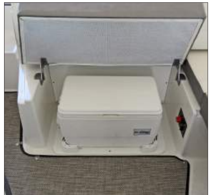
Cooler & Battery Switch Below Bench Seat Cushion
