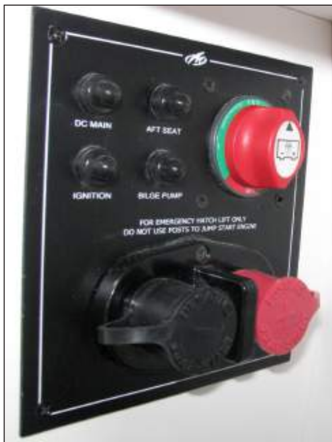
M6 Dual Battery Switch Panel with Circuit Breakers and Engine Hatch Jumper Terminals
