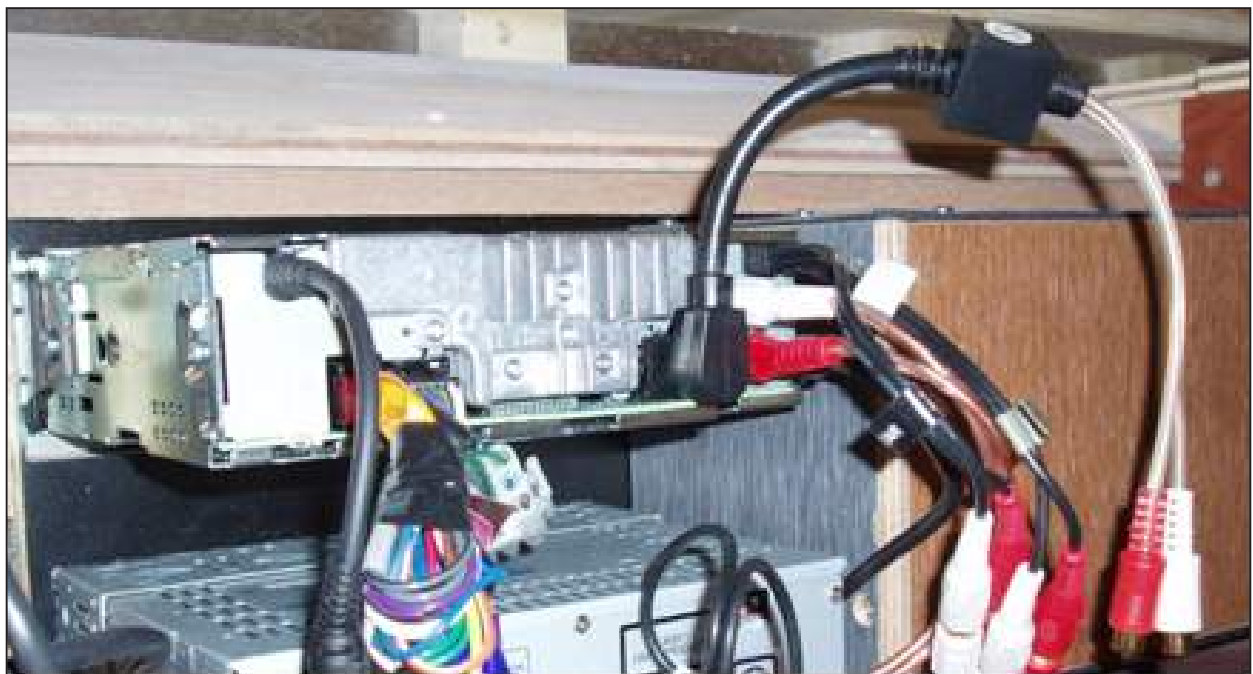
MP3 ADAPTER CONNECTION IF SIRIUS RADIO NOT INSTALLED, PLUG ADAPTER INTO STEREO
