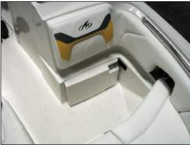
M4 with Bow Lounge Seat Cushion Removed and Foldout Support Latched in the Stored Position
