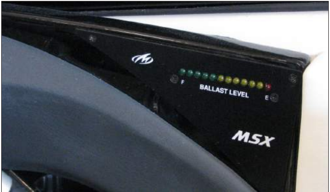
Ballast Tank Level Indicator
