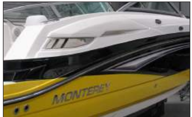
Starboard Engine Compartment Vent
