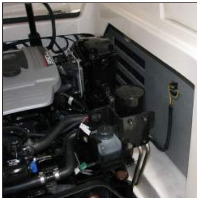
Port Storage Compartment Vents Located in Engine Compartment
