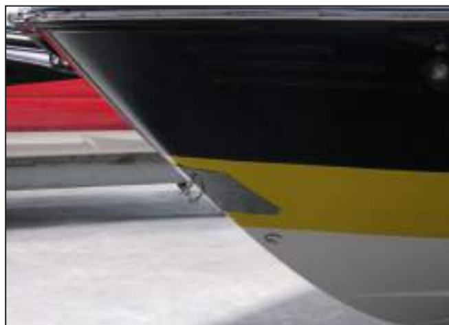
Rope Locker Drain
