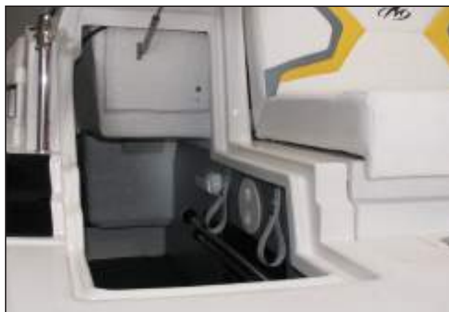
Port Wakeboard Storage Compartment with Through Ventilation to the Engine Compartment
