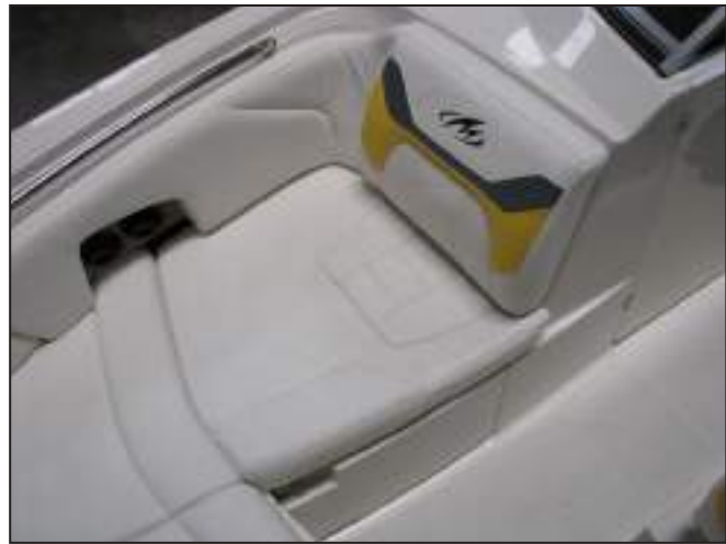
M4 with Bow Lounge Seat Cushion Installed and Foldout Support Latched in the Open, Seat Support Position
