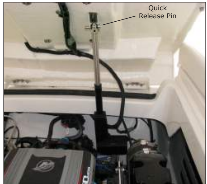
Engine Hatch Actuator and Emergency Quick Release Pin
