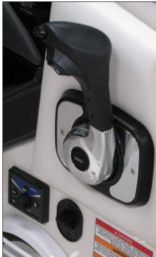
Volvo Side Mount Electronic Control with EVC Panel and Emergency Stop Switch
