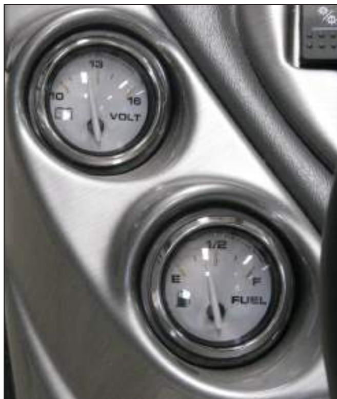
Volt Meter and Fuel Gauge
