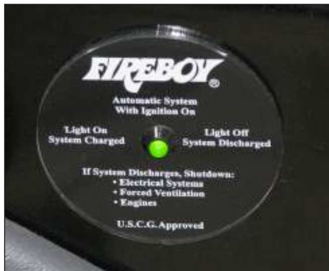
Fire Extinguisher Panel in Helm
