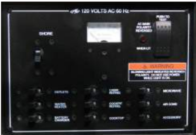
275/295SY AC Circuit Breaker Panel - 120 Volt/60 Hz
