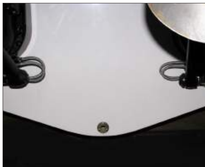
Typical Bilge Drain Plug In Transom
