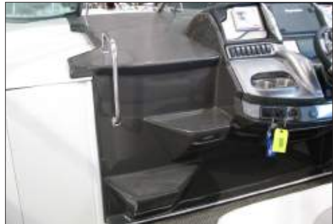
315SY Deck Access Steps Built Into Helm Bulkhead
