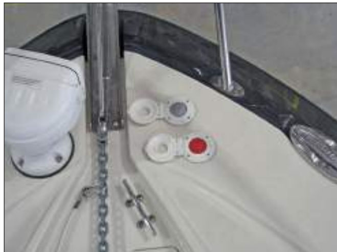
Anchor Line Cleat & UP/Down Deck Foot Switches
