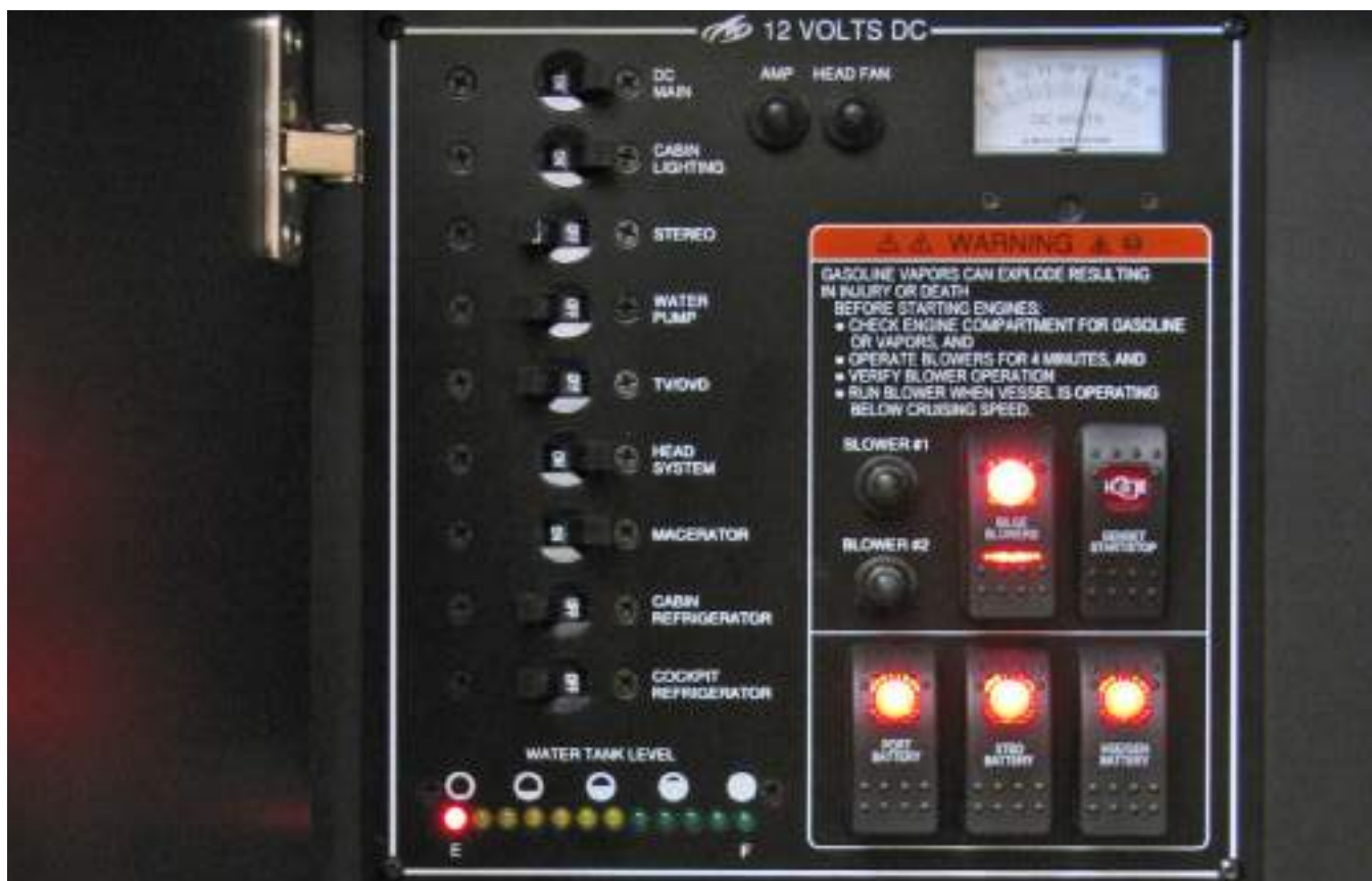
315SY Cabin DC Circuit Breaker Panel, Optional Generator Control Panel & Battery Switch Panel
