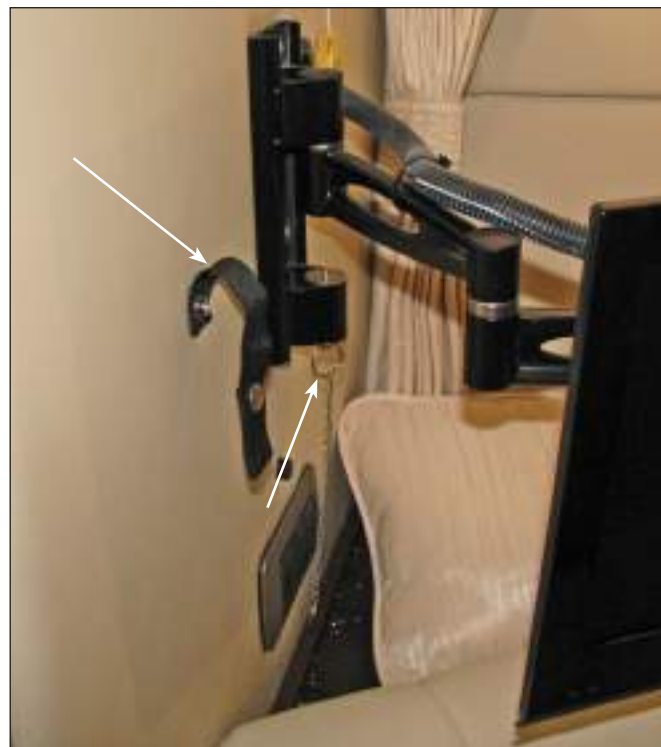
315SY TV Mounting Bracket, Strap & Quick Release Pin
