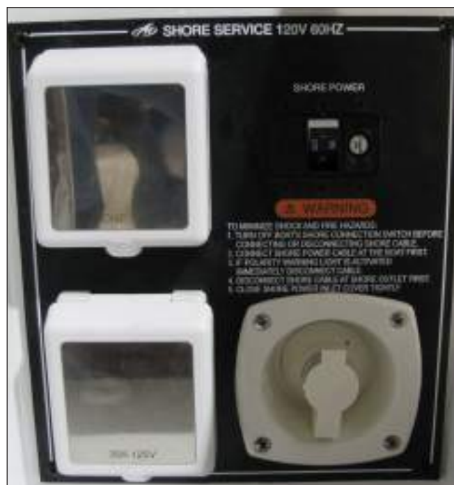
275/295SY 120 Volt Shore Inlet Panel With ELCI
