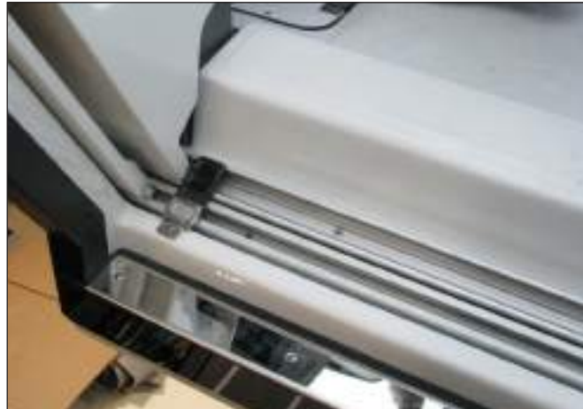
Cabin Door Latched in Open Position
