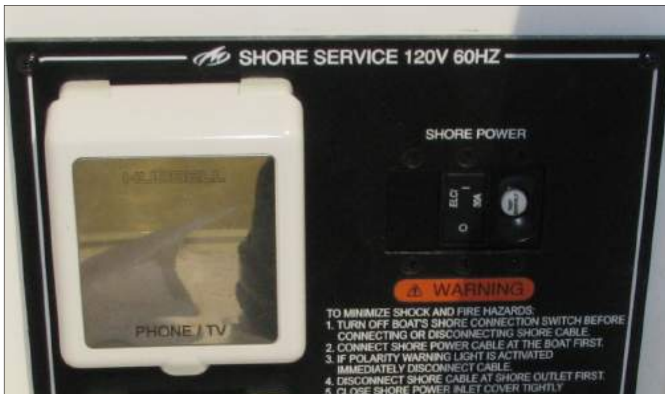
275/295 Inlet Panel ELCI Circuit Interrupter/Circuit Breaker
