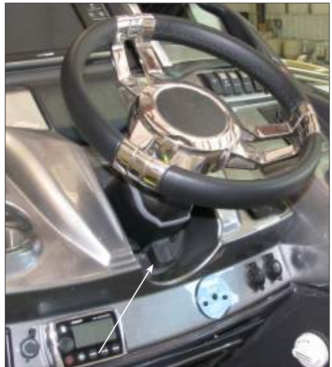
Tilt Steering Wheel & Tilt Release Lever
