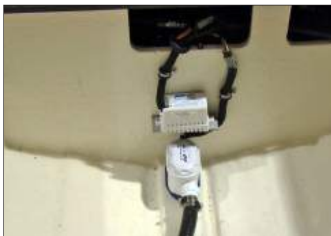
275/295SY Aft Bilge Pump With Built-in Automatic Switch & High Water Alarm/Emergency Pump Float Switch
