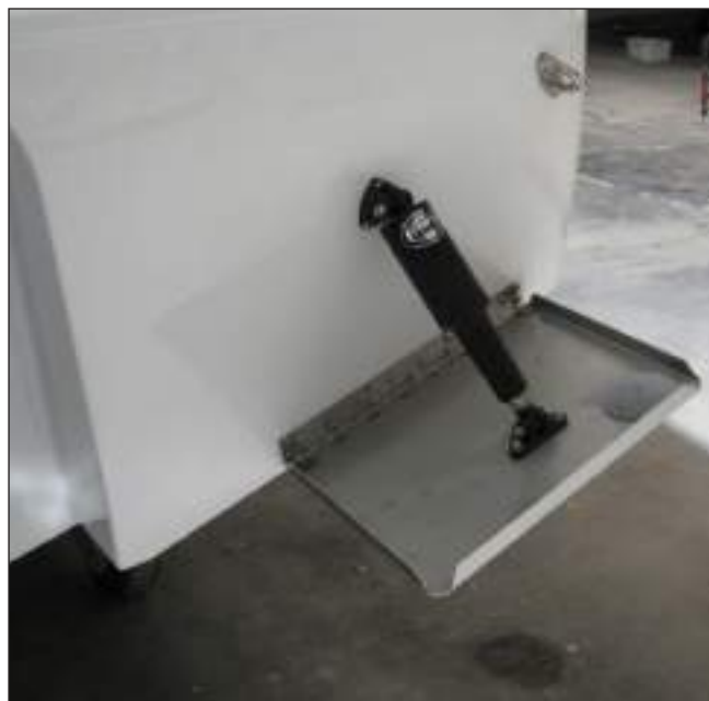
Typical Trim Tab Plane, Actuator & Sacrificial Anode
