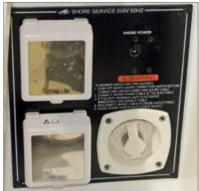
275/295SY 220 Volt AC Inlet Panel With ELCI
