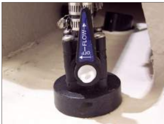
Air Conditioner Seacock (Thru-Hull Valve)
