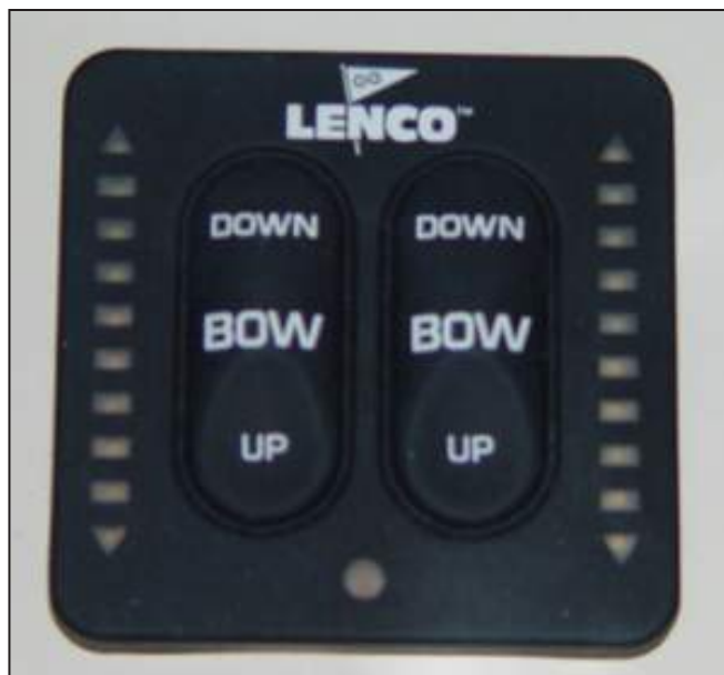
Standard Trim Tab Control Switch Panel
