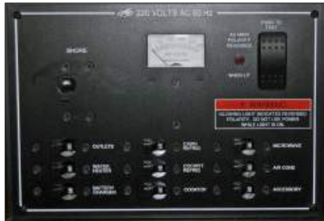
275/295SY AC Circuit Breaker Panel - 220 Volt/50 Hz
