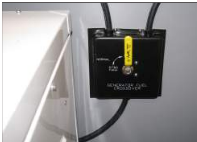
315SY Generator Fuel Tank Selector Valve Port Fuel Tank Selected
