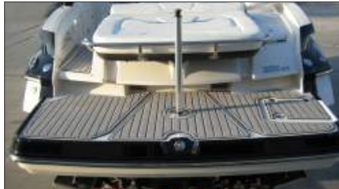
Typical Platform Ski Tow Pylon
