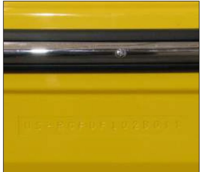
Hull ID # On Starboard Side of Transom
