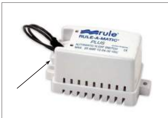
Automatic Float Switch Test Button Push Button Down & Hold Until Pump & Alarm Activate
