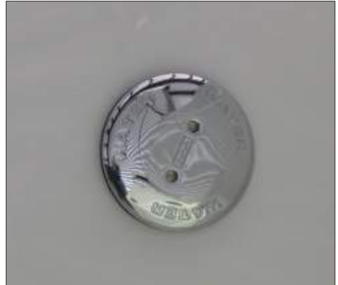
Fresh Water Fill
