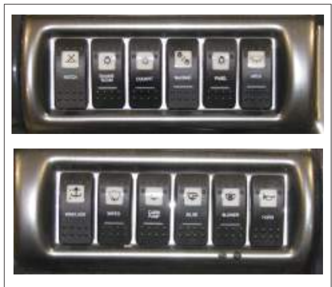
Typical 275SY Helm Switch Panel
