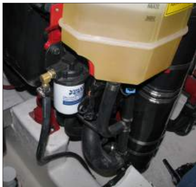
Typical Spin On Engine Fuel Filter
