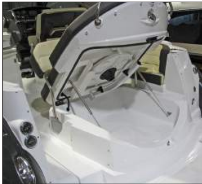
Typical Transom Storage Compartment Below Sun Lounge
