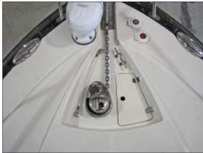
Anchor Rope Locker, Windlass, Anchor Line Cleat, Chain Binder & UP/Down Deck Foot Switches
