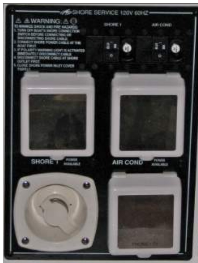
315SY 120 Volt Shore Inlet Panel With ELCI
