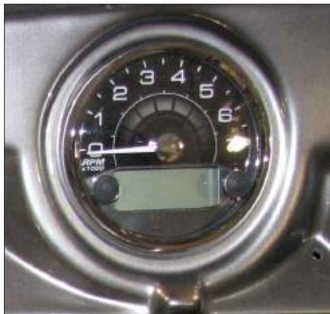
Typical Digital Analog Tachometer & LCD Screen
