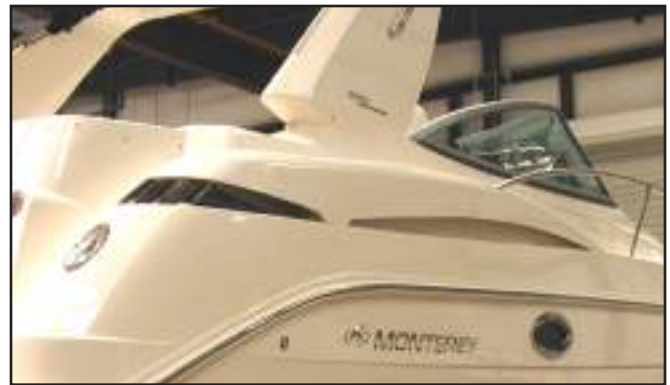
Engine Compartment Vents
