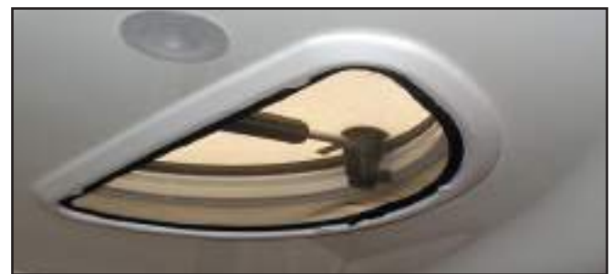
Galley Hatch Fully Closed Screen Installed
