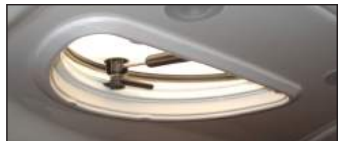
Galley Deck Hatch Secured in Vent Position
