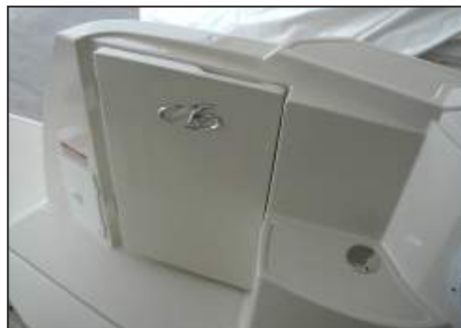
Transom Door in the Open Position (door must be in the open position to open the engine hatch)
