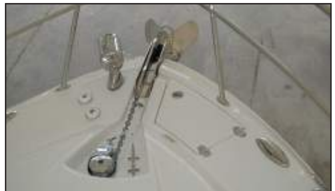
Anchor Locker Hatch, Retractable Cleats, Spot Light, Windlass and Windlass Deck Switches
