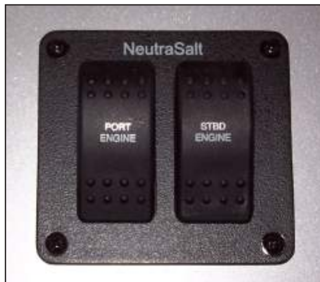
Neutra Salt Switches at Helm
