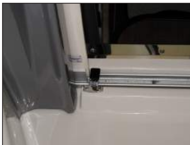
Cabin Door Latched in the Open Position
