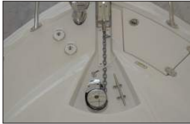
Windlass and Deck Switches
