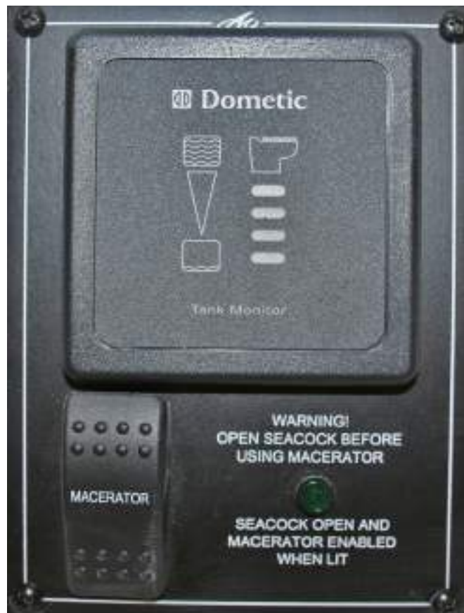
Holding Tank Monitor Panel
