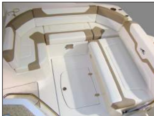
Cockpit Lounge Seat in the Aft Position (the backrest should be in this position whenever the engines are running)
