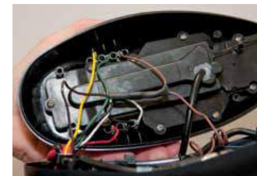
FIGURE 18 Insert AutoPilot wires into terminal holders.
