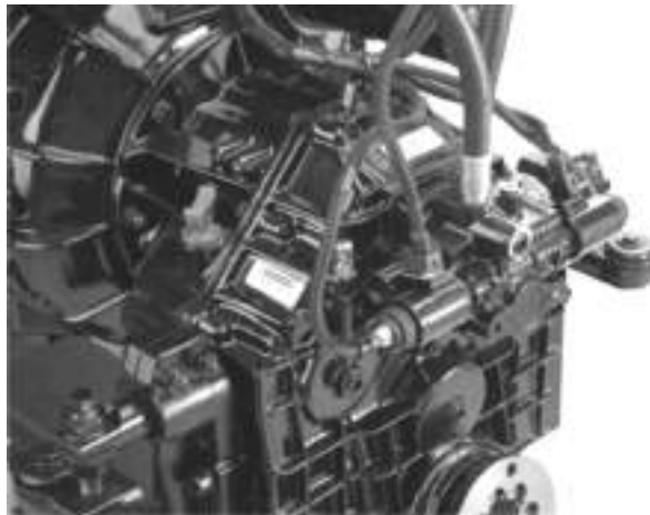
ZF Marine transmission—DTS (oil temperature sensor not installed)
