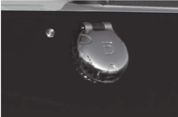
Figure B33: Fuel Deck Fill
