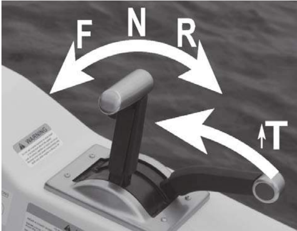
Figure D4: Separate Shift & Throttle Control Operation
