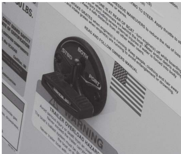
Figure B61: Port/Starboard Ballast Selector Switch
