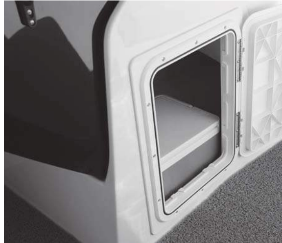
Figure C16: Port Console Storage
