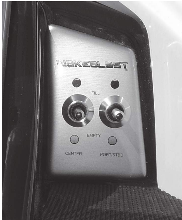
Figure B60: Ballast System Switch Panel
