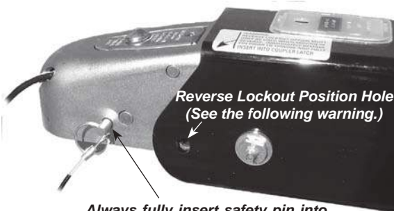
Figure F17: Reverse Manual Brake Lockout
