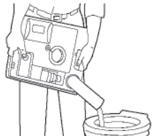
Figure B55: Emptying Waste Holding Tank
