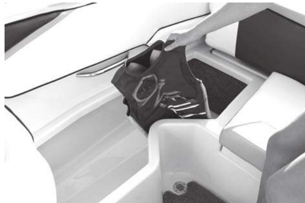
Figure C17: Starboard Cockpit Seat Cushion Storage
