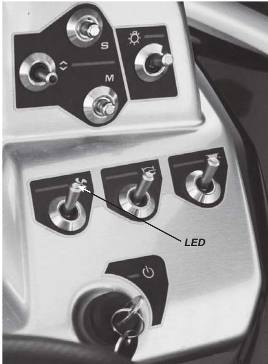
Figure B22: Helm Switches w/LED
