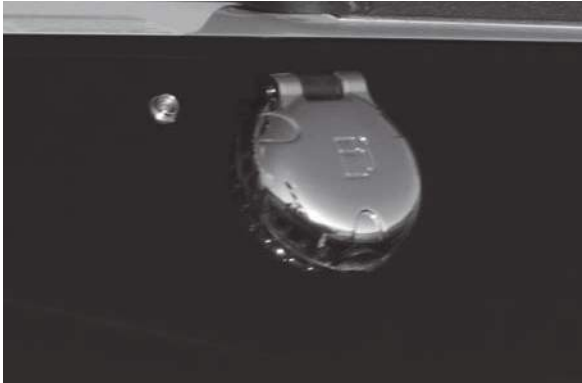
Figure B33: Fuel Deck Fill
