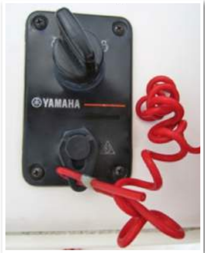
Engine stop switch (above)
