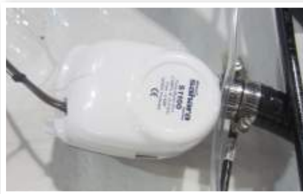
The Bilge Pump is Mounted to ABS Plastic
