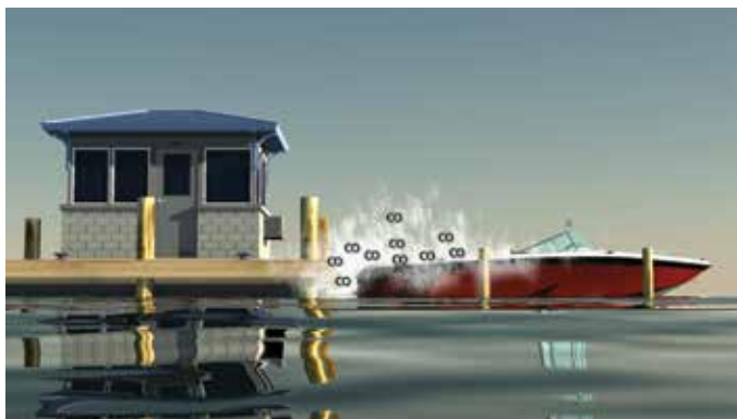
Blockage of boat exhaust by obstruction.
