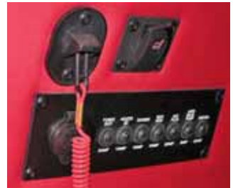
Figure 2-19. Emergency Engine Stop Switch
