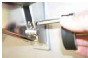
Figure 2-28. Swim Step Pin Removal
