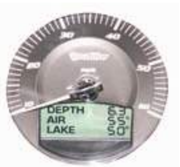
Figure 2-3. Speedometer with Depth, Air and Lake Temperature Gauge
