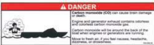
Figure 1-5. Carbon Monoxide Hazards
