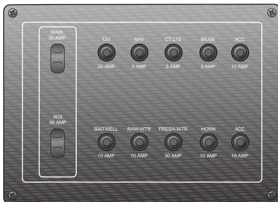
TYPICAL BREAKER / FUSE PANEL
