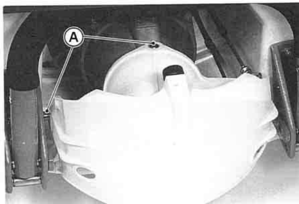
A. Steering Nozzle/Reverse Bucket Pivots
