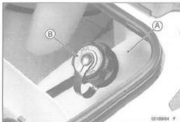
A. Engine Oil Tank B. Oil Filler Cap
