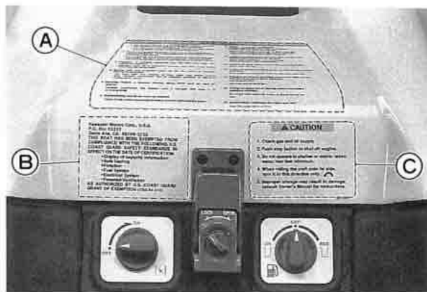
A. Warning B. U.S. Coast Guard Grant of Exemption (US model only) C. Caution
