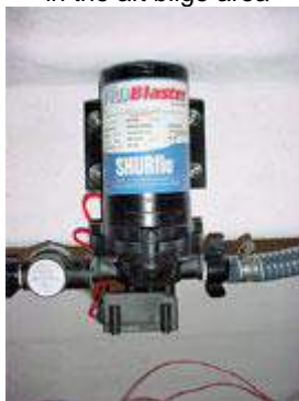
Baitwell pump is located in the aft bilge area
