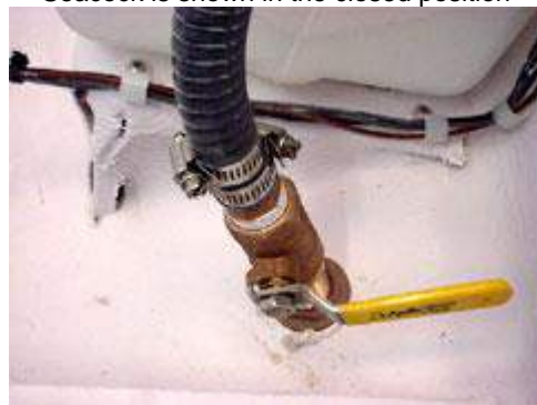
Seacock is shown in the closed position
