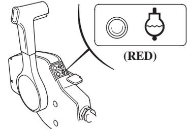
If the engine overheats, the red light will come on, and the engine protection system will limit engine speed.
