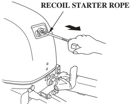
Inspect the recoil starter rope, and replace it if it becomes frayed.
