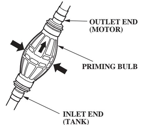
A priming bulb is built into the fuel hose that connects the fuel tank to the outboard motor.
