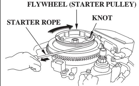
5. Pull the emergency starter rope slowly until resistance is felt, then pull briskly.
