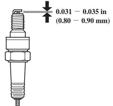
5. Measure the spark plug electrode gap with a suitable gauge. The gap should be 0.031 - 0.035 inches (0.80 - 0.90 mm).
