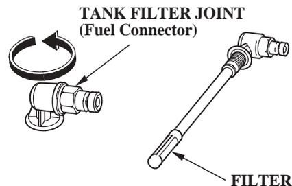
1. Unscrew the fuel hose connector by turning it counterclockwise, then remove the fuel hose connector and fuel filter from the tank.
