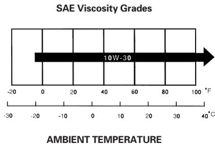
SAE 10W-30 is recommended for general use. Other viscosities shown in the chart may be used when the average temperature in your area is within the recommended range.
