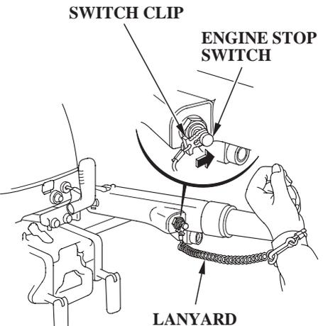
1. Put the emergency stop switch clip in the engine stop switch, and attach the lanyard to your PFD (Personal Flotation Device) or to your wrist, as shown.
