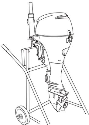
Store the outboard motor either vertically or horizontally with the tiller handle side up.
