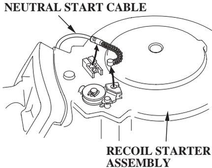
2. Move the shift lever to the F (forward) position. Loosen the neutral start cable lock nut and disconnect the neutral start cable. Unscrew the three bolts and remove the recoil starter assembly.
