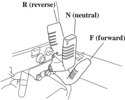
To shift gears, turn the throttle grip to the SLOW position, then move the gearshift lever to select F (forward), N (neutral) or R (reverse) gears.
