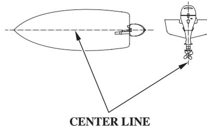
Install the outboard motor on the center of the boat transom.
