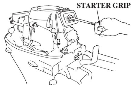
4. Remove the spark plugs (p. 61 ), and remove the clip from the emergency stop or engine switch. Pull the recoil starter grip, rotate the flywheel a few revolutions to completely expel any water from the cylinders.
