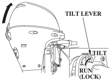
The tilt lever enables the outboard motor to be raised for shallow water operation, beaching, launching, or mooring.
