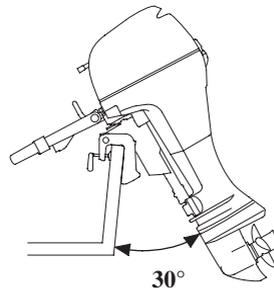
To tilt the outboard motor, move the tilt lever to the TILT position, then raise the outboard motor to the 30° or 45° position by pulling on the engine cover grip.
