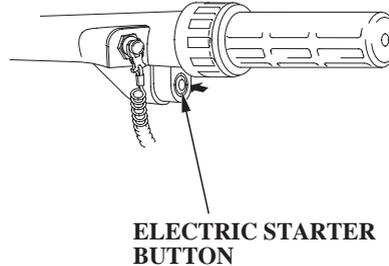
Press the starter button to operate the electric starter for starting the engine.
