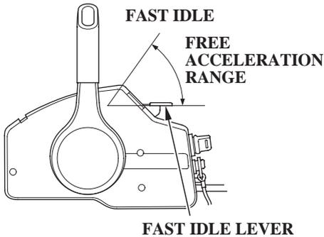
3. To start a cold engine, leave the fast idle lever in the OFF (fully lowered) position.
