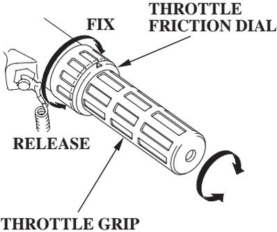
Use the throttle friction dial to help hold a constant throttle setting while cruising.
