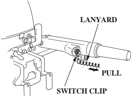
To stop the engine in an emergency, pull the clip out of the engine or emergency stop switch by pulling the lanyard.
