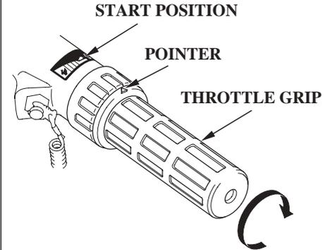
4. Do not turn the throttle grip before starting and align the START position with the pointer for starting the engine.
