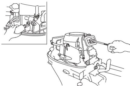
5. Pour a teaspoon of engine oil into each spark plug hole, then pull the recoil starter grip several times to lubricate the inside of the cylinders.
