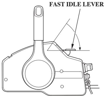
5. If the fast idle lever was used to start the engine, gradually lower the lever as the engine warms up.
