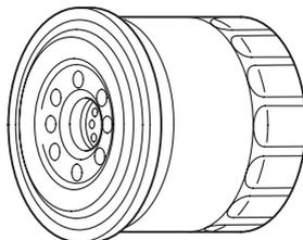
4. Clean the oil filter mounting base, and coat the gasket of the new oil filter with clean engine oil.
