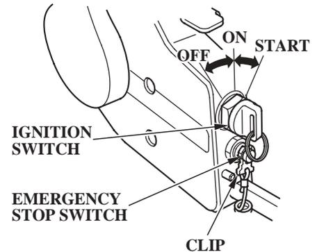
The ignition switch controls the ignition system and starter motor.
