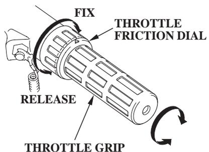
The throttle friction dial adjusts resistance to throttle grip rotation.
