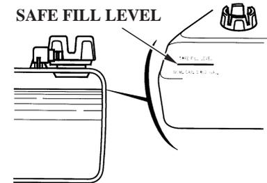
Refuel in a well-ventilated area. Fill the tank to the SAFE FILL LEVEL line.
