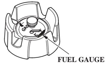
A fuel gauge is built into the cap of the portable fuel tank.
