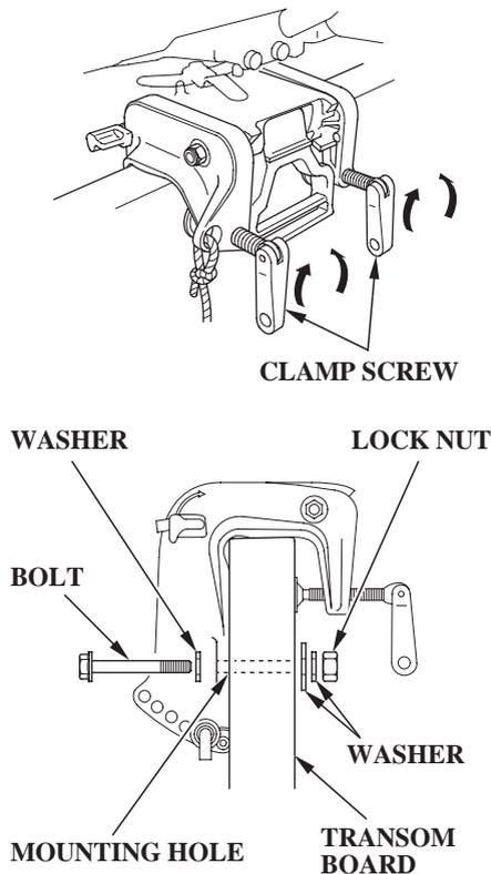
Attach the stern bracket to the boat transom by tightening the clamp screws.
