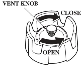
The cap is provided with a vent knob to seal the portable fuel tank for carrying it to and from the boat. Open the vent knob 2 or 3 turns before starting the engine ( p. 34 ).
