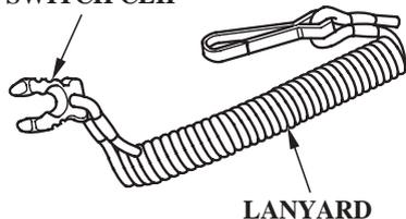
The engine stop switch has controls for normal engine stopping and emergency engine stopping.
