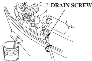
2. With the outboard motor in a vertical position, place an approved gasoline container below the fuel drain outlet, and use a funnel to avoid spilling fuel. Loosen the drain screw to drain fuel from the carburetor.
