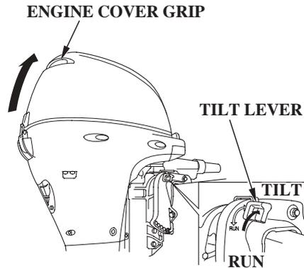
To return the outboard motor to the normal operating position, move the tilt lever to the RUN position, raise the outboard motor slightly to disengage the tilt mechanism, then slowly lower the outboard motor.
