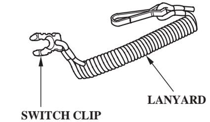
The switch clip must be inserted in the emergency stop switch in order for the engine to start and run. The lanyard must be attached to the operator's PFD (Personal Flotation Device) or worn around the wrist as shown.
