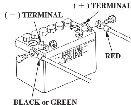
Connect the positive (+) battery cable to the positive (+) battery terminal, then connect the negative (-) battery cable to the negative (-) battery terminal.
