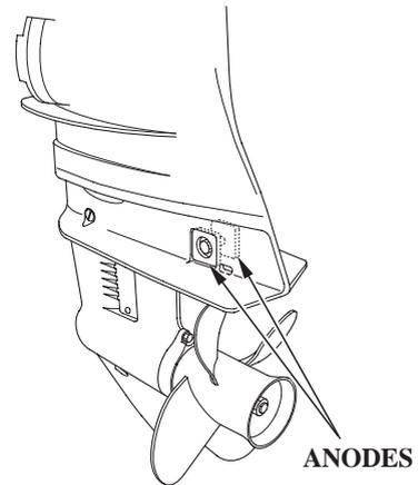
The anodes are made of a sacrificial material that helps to protect the outboard motor from corrosion.
