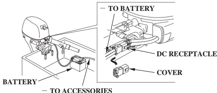
To prepare the outboard motor for connection to a battery, pull the cover out of the DC receptacle, connect your battery charging wires to the receptacle. Attach the connected DC receptacle on the holder on the tiller arm.
