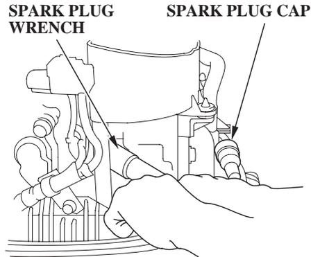
4. Inspect the spark plugs. Replace them if the electrodes are worn, or if the insulators are cracked or chipped. Clean the spark plugs with a wire brush if you are going to reuse them.
