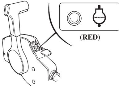
If the engine overheats, the red indicator light will come on, and the engine protection system will limit engine speed. If you are at cruising speed, engine speed will decrease gradually.
