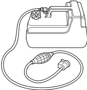
Place the portable fuel tank in a well-ventilated location, away from direct sunlight, to reduce the possibility of a gasoline vapor explosion.
