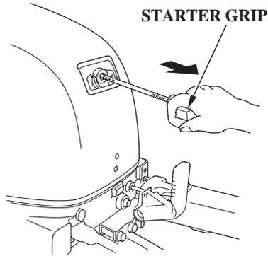
Pull the starter grip to operate the recoil starter for starting the engine manually.
