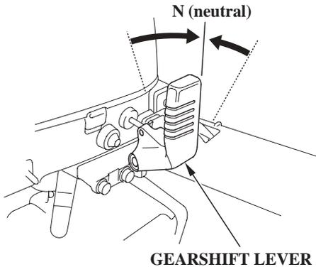
2. Check the position of the gearshift lever. It must be in the N (neutral) position for starting.
