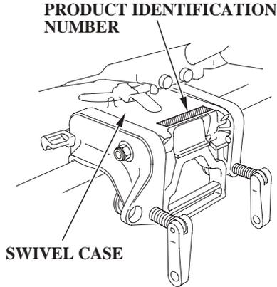
The product identification number is stamped on a plate attached on top of the stern bracket.
