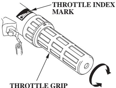
The throttle grip controls engine speed.
