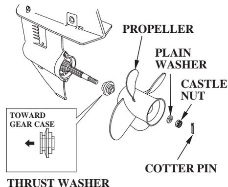
1. Install the propeller in the reverse order of removal.
