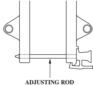
Proper adjustment prevents the outboard motor from being trimmed too low (p. 48 ).
