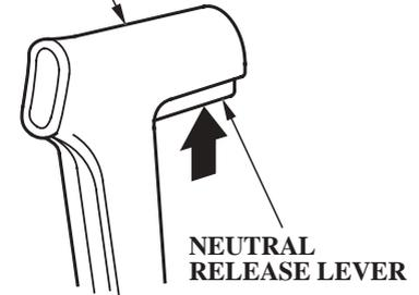
The control lever automatically locks itself in the N (neutral) position. To move the lever out of the N (neutral) position, you must squeeze the neutral release lever on the underside of the lever handle.
