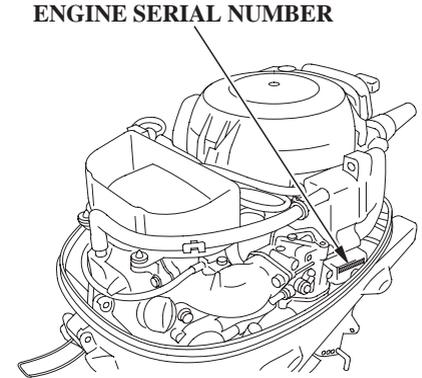
The engine serial number is stamped on the right front of the engine.
