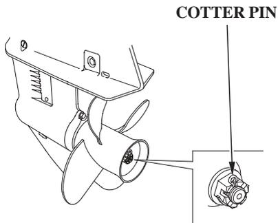
Remove the coter pin, unscrew the castle nut, remove the washer, then remove the propeller and thrust washer.
