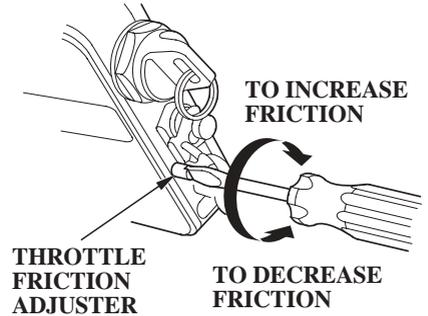
Adjust the throttle friction adjuster so the control lever will hold a constant throttle setting while cruising.
