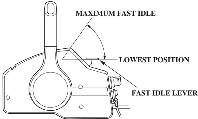
The fast idle lever is provided with the engine idle speed adjusting function.
