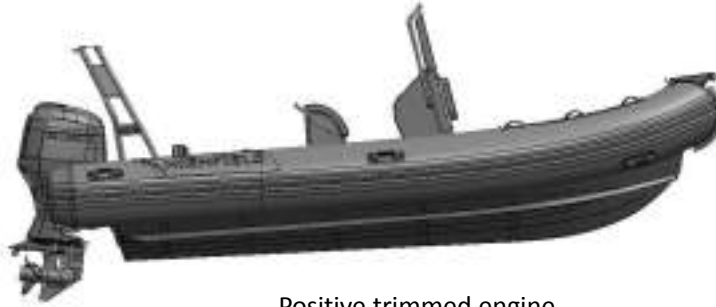
Positive trimmed engine
