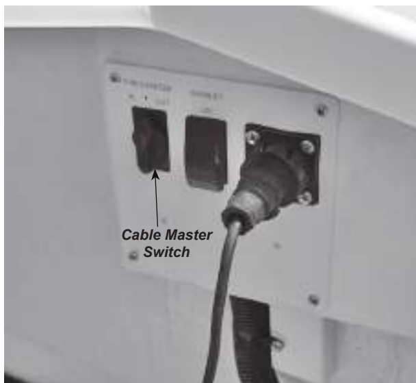
Figure H26: Cablemaster Switch Location
