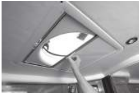
Figure K1: Layered Deck Hatch Screen/Sun/Shade System
