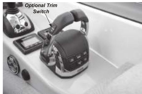
Figure F3: Volvo Penta's Dual Binnacle Control w/Trim (Trim Switch - Stern Drive Models Only)
