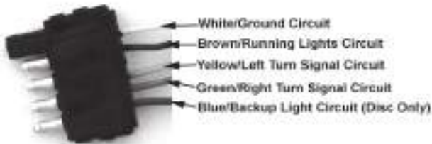
Figure S6: 5-Wire Plug Harness
