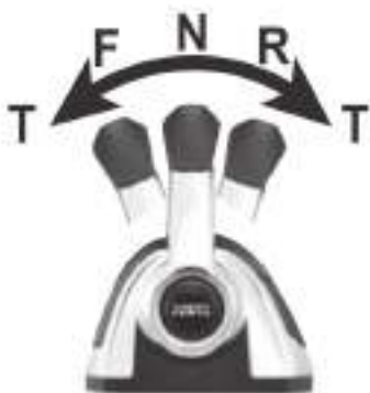
Figure F5: Control Lever Positions - Dual Binnacle (Representative View - Models may vary)
