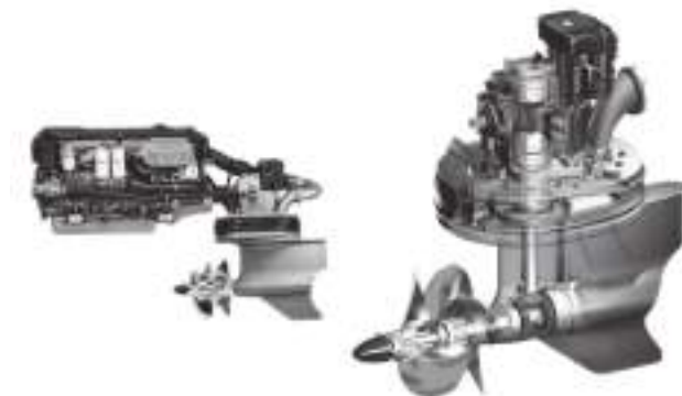
Figure E2: Volvo Penta IPS Drive-Unit
