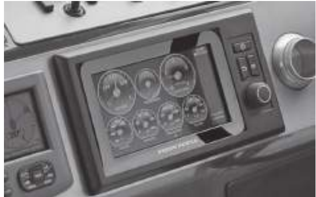
Figure E6: EVC System Display Panel (Representative View - Models May Vary)
