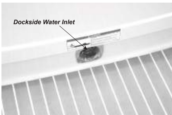
Figure J8: Dockside Water Inlet
