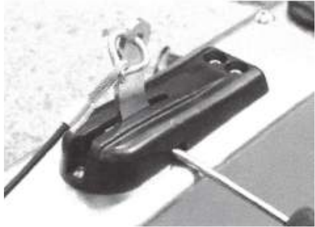
Figure S15: Pry Up w/ Screwdriver on Spring Plate
