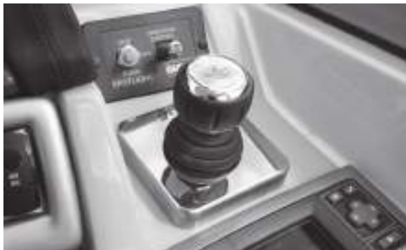
Figure F7: MerCruiser's "Axis" Joystick
