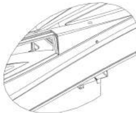
Figure I14: Port Fuel Vent Location (Port & Stbd Typical)
