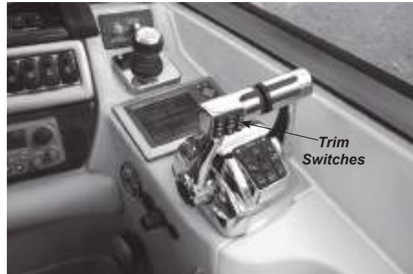
Figure F2: Mercruiser's Dual Binnacle Control w/Trim (Trim Switches - Stern Drive Models Only)
