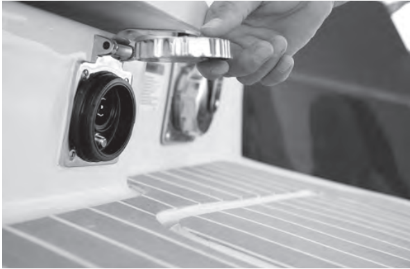
Figure L18: Phone/Cable TV Dockside Inlet Location
