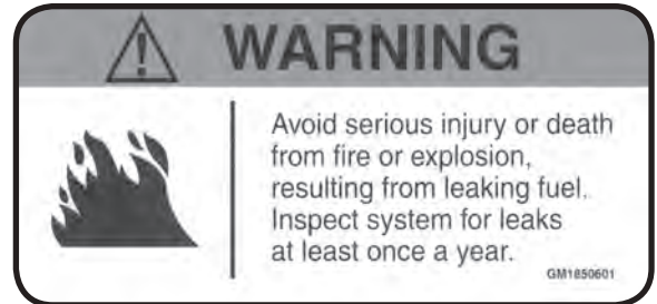
Leaking Fuel Warning Label
