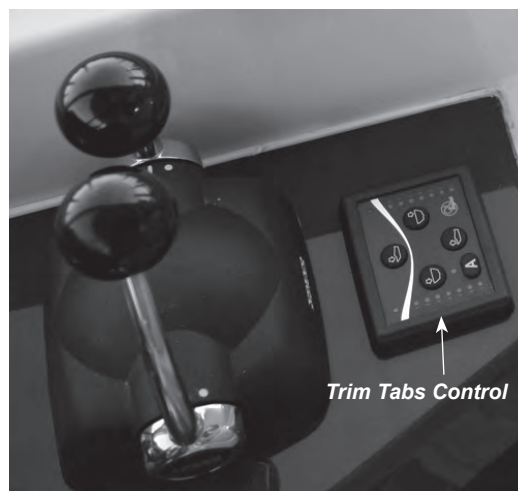
Figure E6: Control Panel - Trim Tabs
