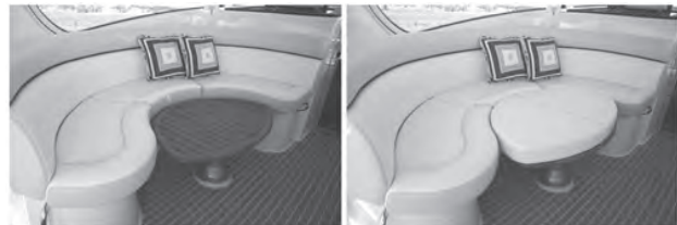
Figure N23: Port Lounge Converted to Berth
