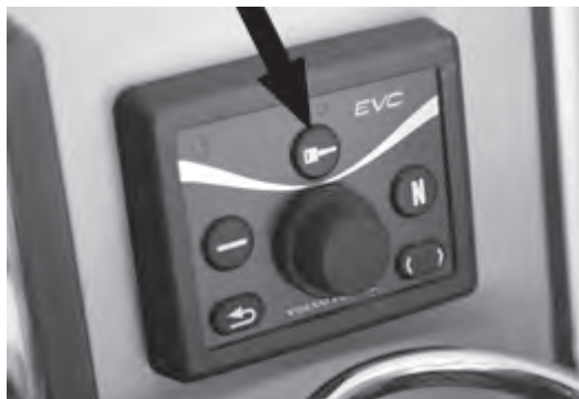
Figure A4: EVC Control Panel Activation Button
