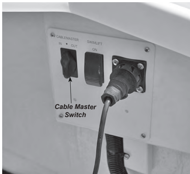
Figure H19: Cablemaster Switch Location
