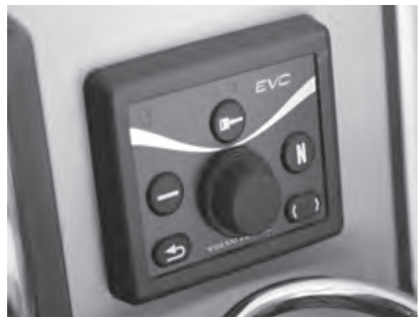
Figure E11: EVC Control Panel
