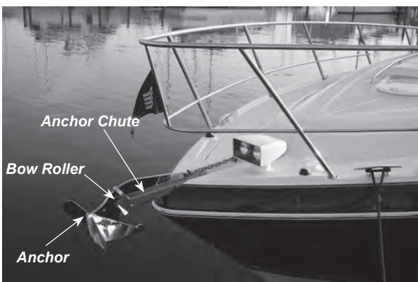
Figure M16: Integrated Bow Platform
