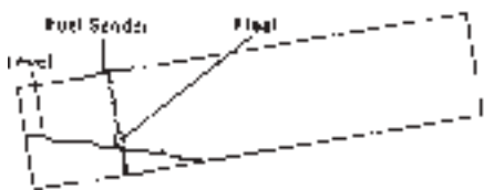
Figure I10: Trim Angle Effect with Low Fuel
