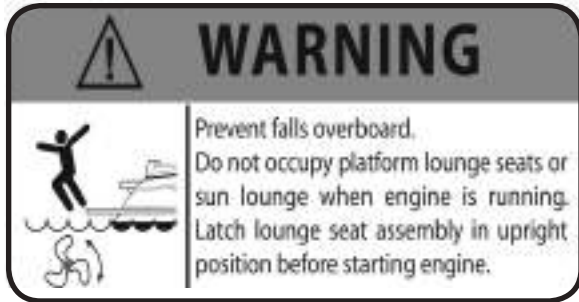
Platform Lounging Seats & Sun Lounge Warning Label
