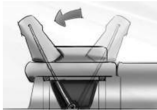
Figure N4: Port & Stbd Seat Backrests (Rotates Forward to Create Passenger's Lounge) (Representative View - Models May Vary)
