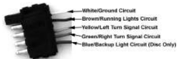
Figure S8: 5-Wire Plug Harness
