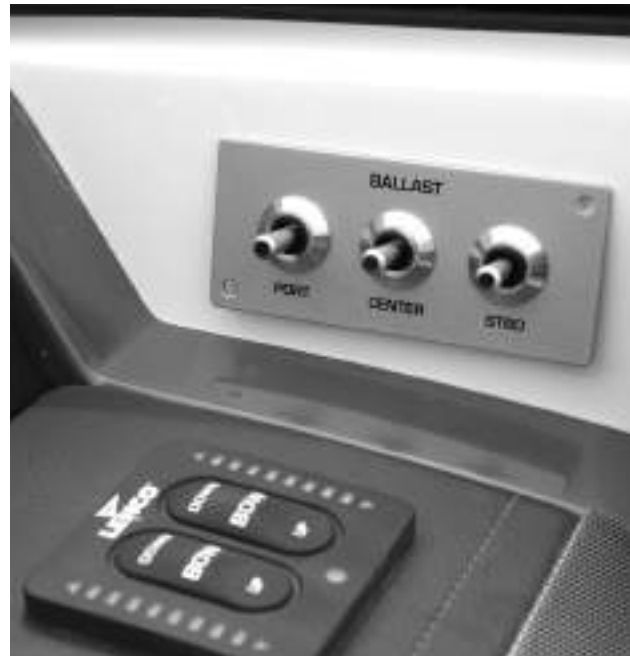
Figure L16: Ballast System Switch Panel
