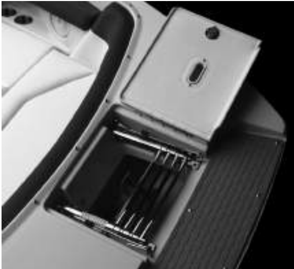
Figure L5: Anchor Locker w/Hidden Ladder
