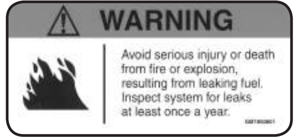
Leaking Fuel Warning Label
