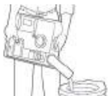
Figure J11: Emptying Waste Holding Tank
