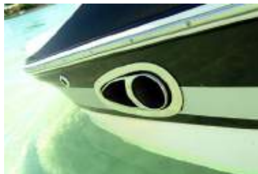
Figure M10: Thru-Hull Exhaust
