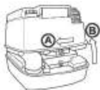
Figure J10: Removing Fresh Water Tank
