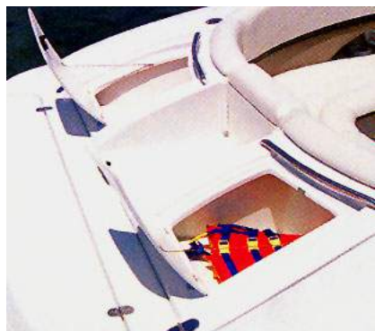
Figure L11: Transom Storage Locker - Dual
