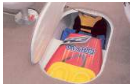
Figure L8: In-Floor Ski Locker
