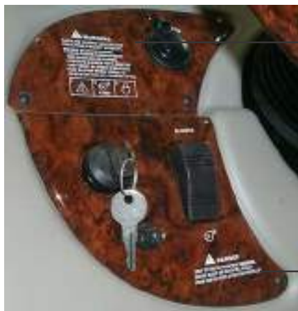
Imprinted Labels on Port Ignition Panel
