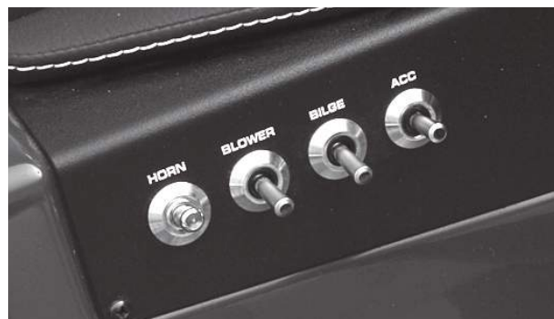
Figure H6: Helm Switch Panel - Port View
