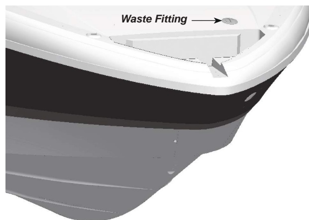
Figure J13: Pumpout Waste Deck Fitting (Location May Vary Depending on Model)
