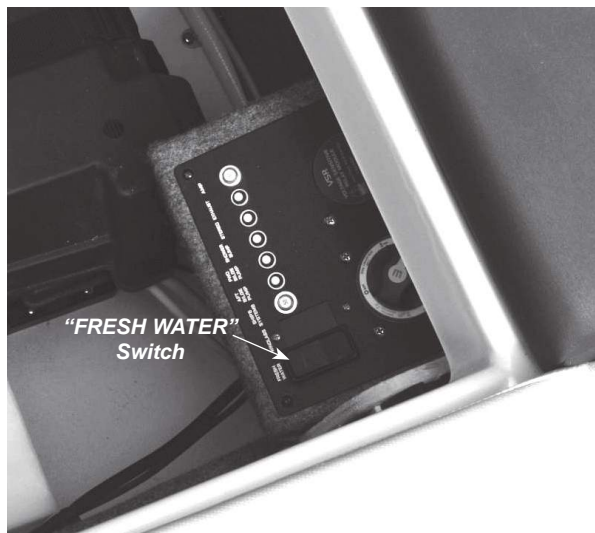
Figure J4: Fresh Water Switch Location (Location May Vary Depending on Model)
