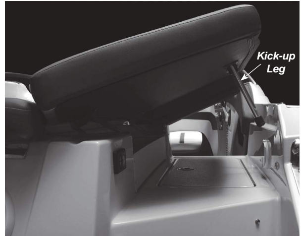
Figure N16: Starboard Sundeck Cushion (Converts to Chaise Lounge - Models May Vary)
