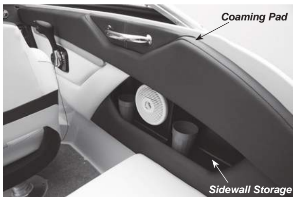
Figure N18: Stbd Coaming Pad with Sidewall Storage (Representative View - Models May Vary)
