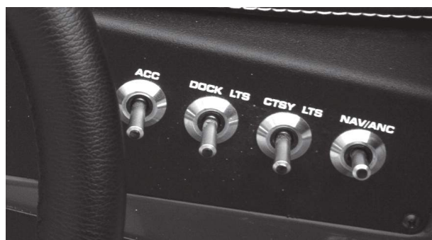
Figure H7: Helm Switch Panel - Starboard View
