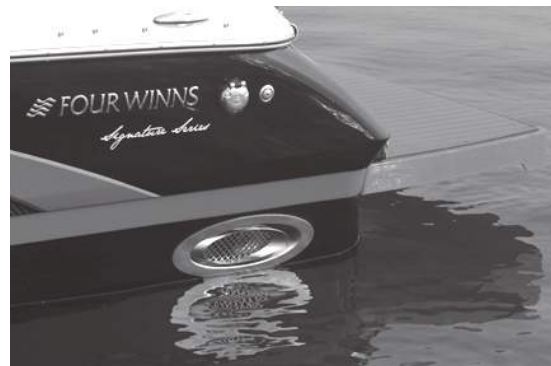
Figure M16: Thru-Hull Exhaust
