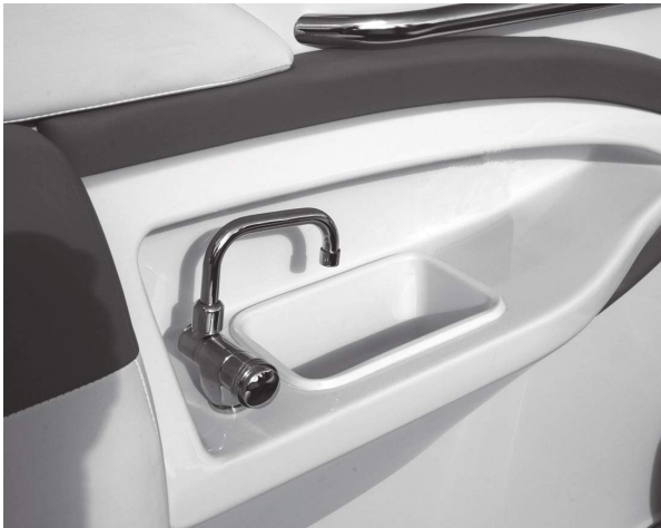
Figure L1: Sink & Faucet - Coaming Pad
