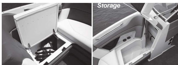
Figure N2: Hinged Bow Cushions (Port & Starboard) (Representative View - Models May Vary)
