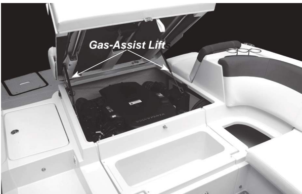
Figure N11: Engine Hatch w/Gas-Assist Lifts (Representative View - Models May Vary)
