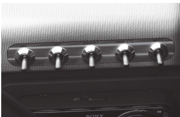
Figure H9: Helm Switch Panel - Starboard View
