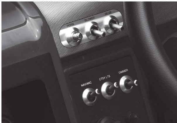
Figure H8: Helm Switch Panel - Port View
