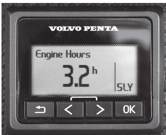
Figure E11: Hour Meter Feature (EVC Engine - Certain Models Only)
