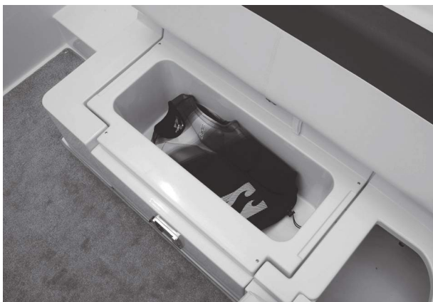
Figure L14: Storage Under Stern Seat Cushions
