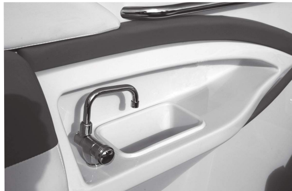
Figure J3: Sink & Faucet - Coaming Pad
