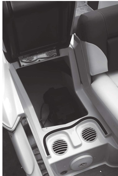
Figure L11: Port Aft Deck Storage Locker To Access: Lift Up on the Port Transom Seat (if applicable). (Note: Certain Models Only - Models May Vary)
