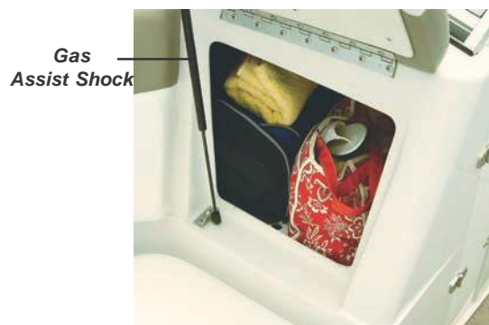
Figure L11: Starboard Helm Console Storage
