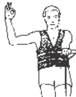
SPEED OK- Arm upraised with thumb and index finger joined to form circle.
