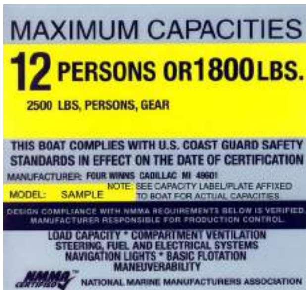
G. SAMPLE - Capacity Label (See Actual Capacity Plate Affixed to Boat for Actual Capacities.
