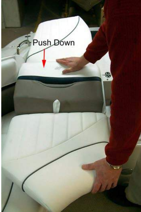
Figure N30: Sun Lounge - Leveling Pad
