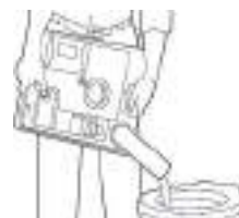
Figure J10: Emptying Waste Holding Tank
