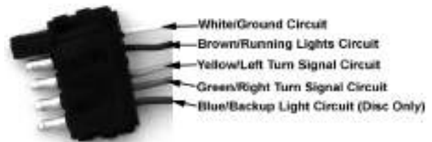
Figure S8: 5-Wire Plug Harness
