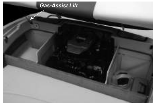
Figure N21: Raised Center Sundeck (One-Piece) - Engine Compartment Access (Representative View - Models May Vary)
