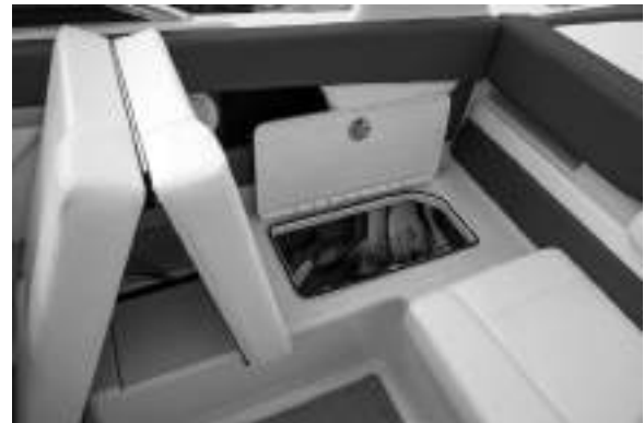
Figure L13: Starboard Cushion Storage (Note: Cushion is hinged to fold up out of the way)
