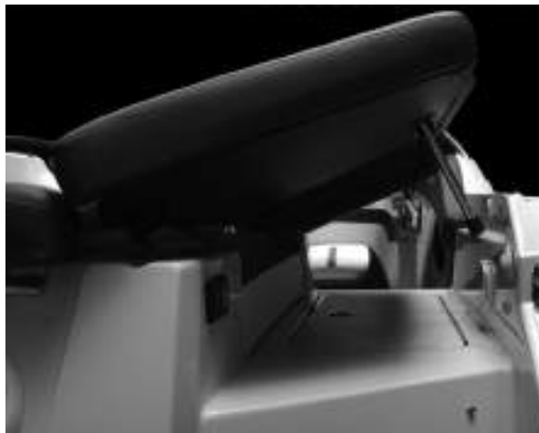
Figure N23: Starboard Sundeck Cushion (Converts to Chaise Lounge - Certain Models Only)
