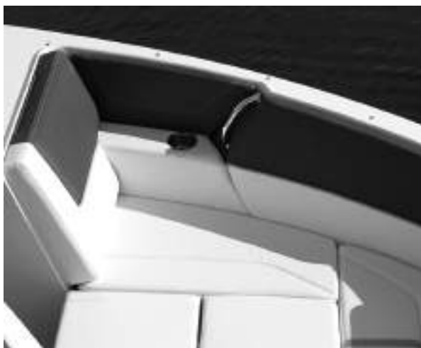
Figure M2: Passenger Assist Handle - Bow (Representative View - Models & Locations May Vary)
