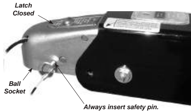
Figure S6: Brake Actuator & Coupling Assembly - Closed (Certain Models Only - GVWR -7000# or less)
