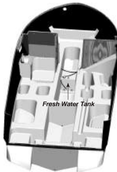
Figure J4: Fresh Water Tank Location (In-Floor Locker)
