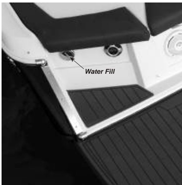
Figure J1: Water Fill - Port Transom
