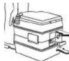
Figure J-8: Porta Potti Bellows Flush Operation
