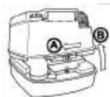
Figure J-9: Removing Fresh Water Tank
