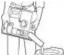
Figure J-10: Emptying Waste Holding Tank
