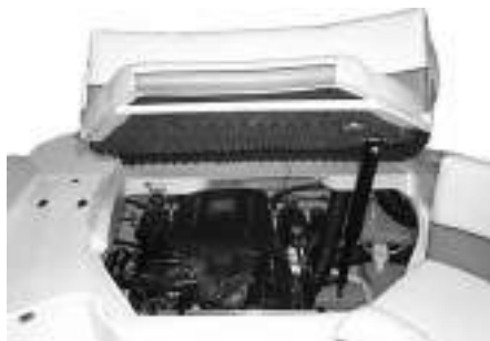
Figure N-8: Electric Motorhood Lift
