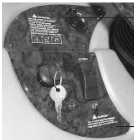
Imprinted Labels on Ignition Panel
