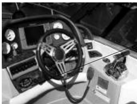
Gasoline Vapors - Blower Warning Label
