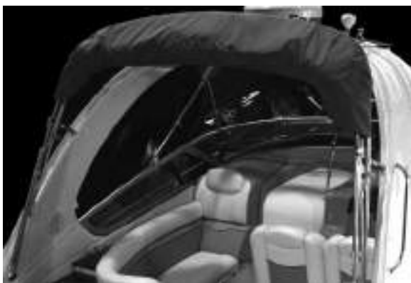
Figure O1: Vista Camper Top - Booted (Representative View)
