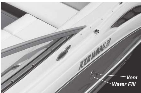
Figure J1: Water Fill
