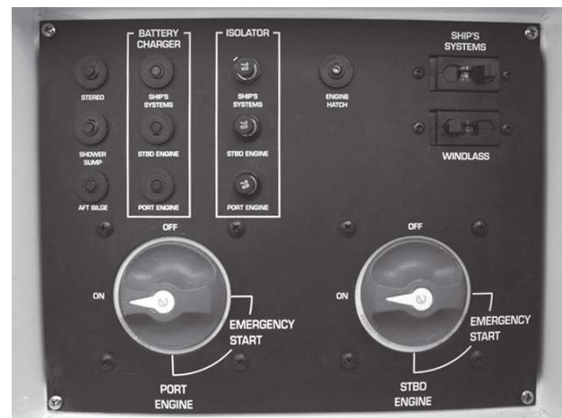
Figure H3: Battery Switch - Twin Engine
