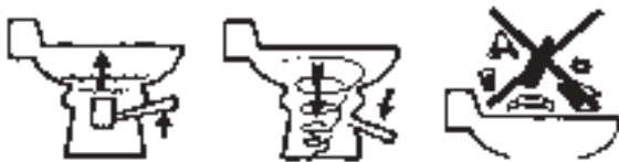
Figure J9: VacuFlush Operations
