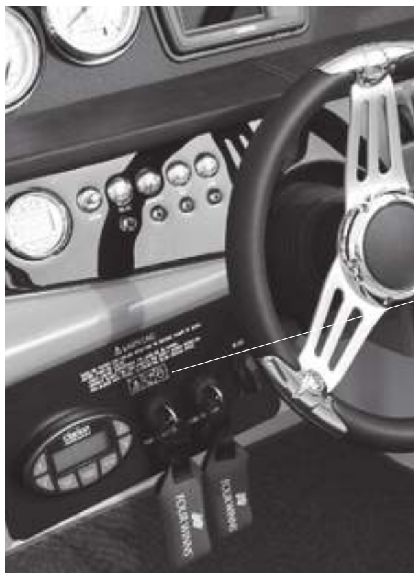
Imprinted Label on Ignition Panel
