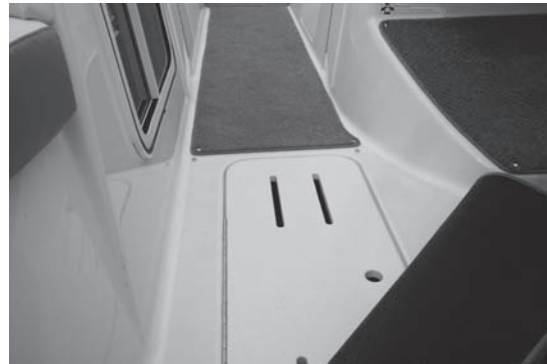
Figure L11: In-Floor Storage Locker
