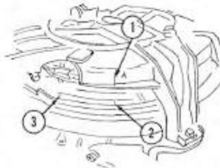
Fig. Mc116 — Manual starting Royal Scott motor showing timing marks. Other two cylinder models are similar.
