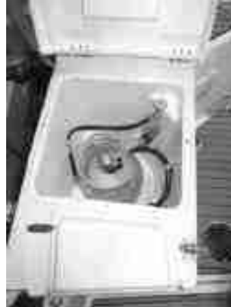
Gas cylinder locker
