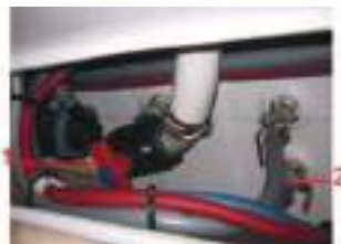
1. WC evacuation to sea 2. Seawater inlet WC
