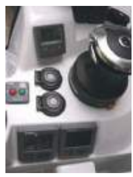
Electric winch - Contactors Genoa sheets
